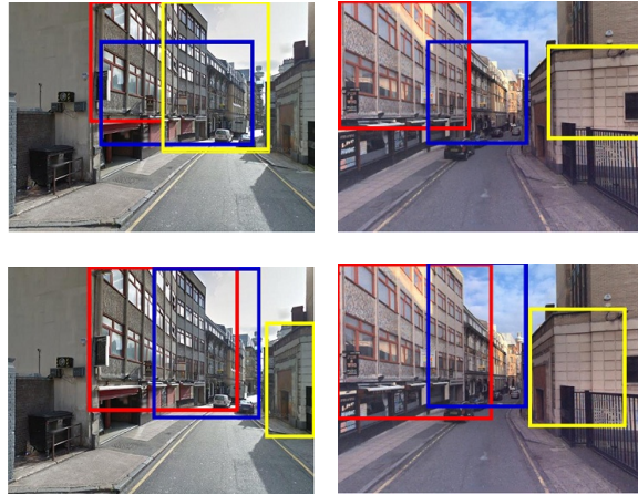
Fig. 7. Use of the view vanishing point to center panoramic sections improves matching of landmarks (bottom) over that obtained using the image center (top).
