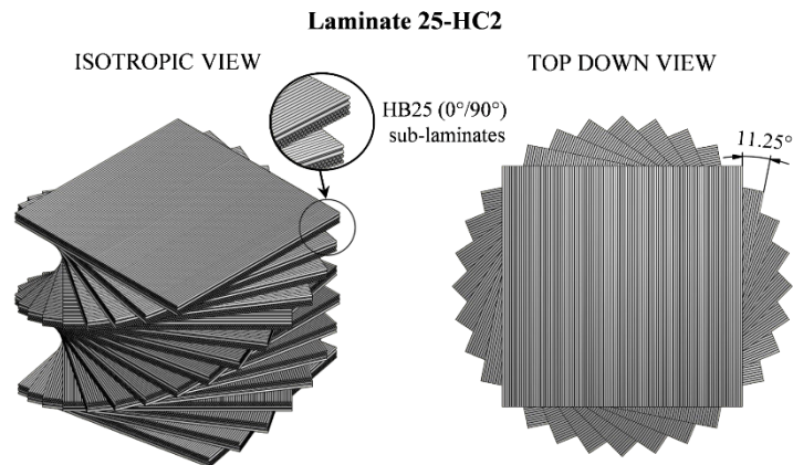
Fig. 3. Example schematic of helicoidal layup 25-HC2 with a sub-laminate angle mismatch of 11.25°. Note that the smaller the angle mismatch of the sub-laminates, the more closely related to [0°/90°] they become.
