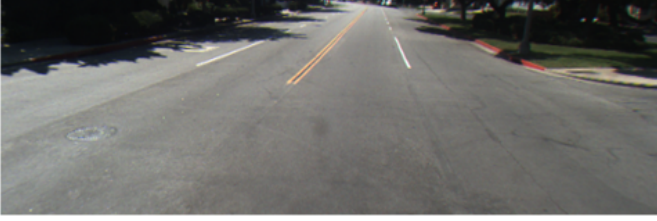
Fig. 5: Example road image with a lack of lane painting in the near field
