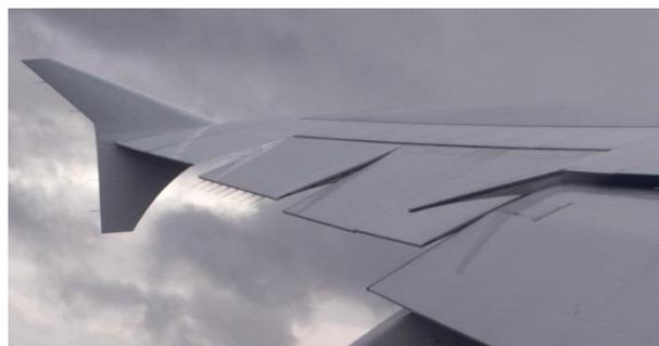
Figure 1. Airbus A380 wing with multiple control surfaces deflected showing the large gaps created.[3]
