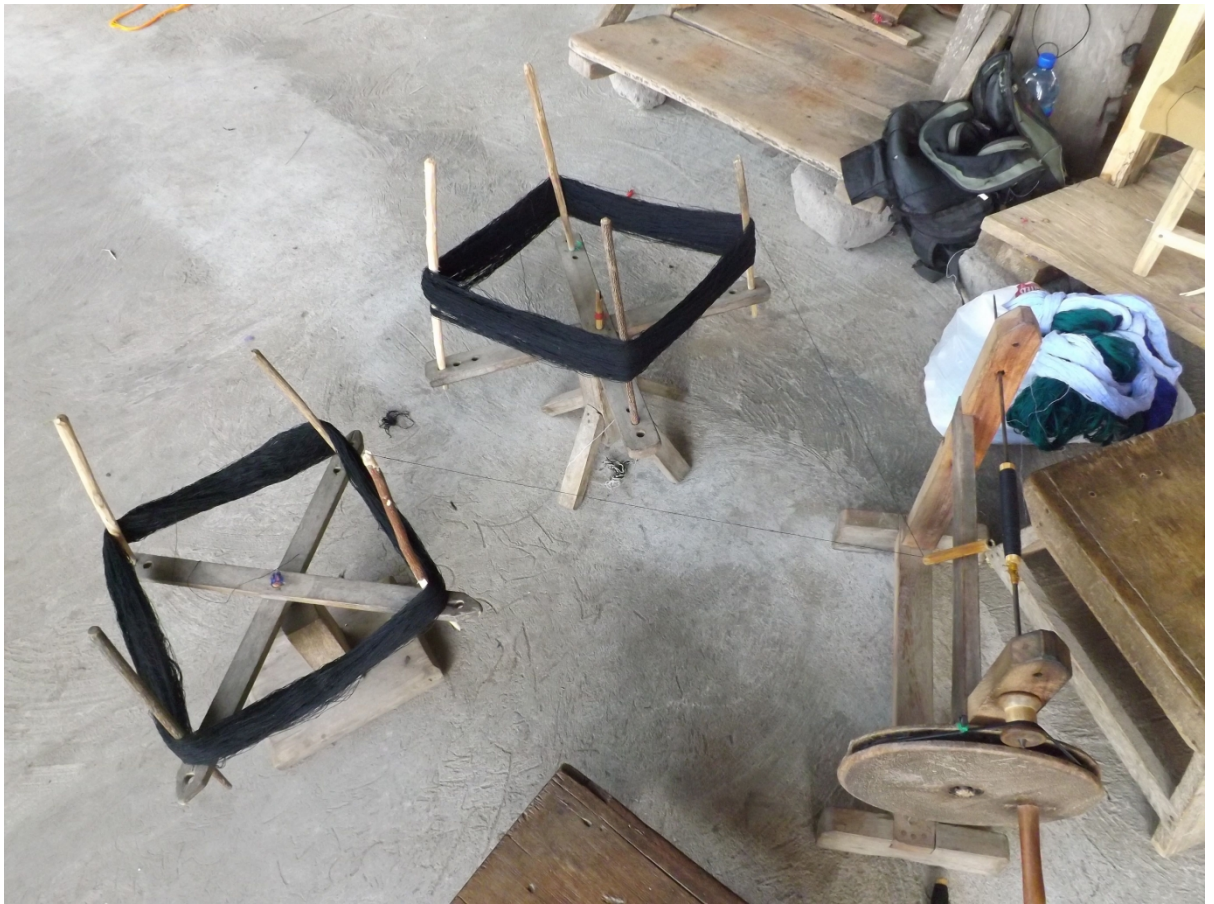
Plate 6- Skein holder machine with cotton yarn and bobbin winder, October 2012. Photograph by author.
