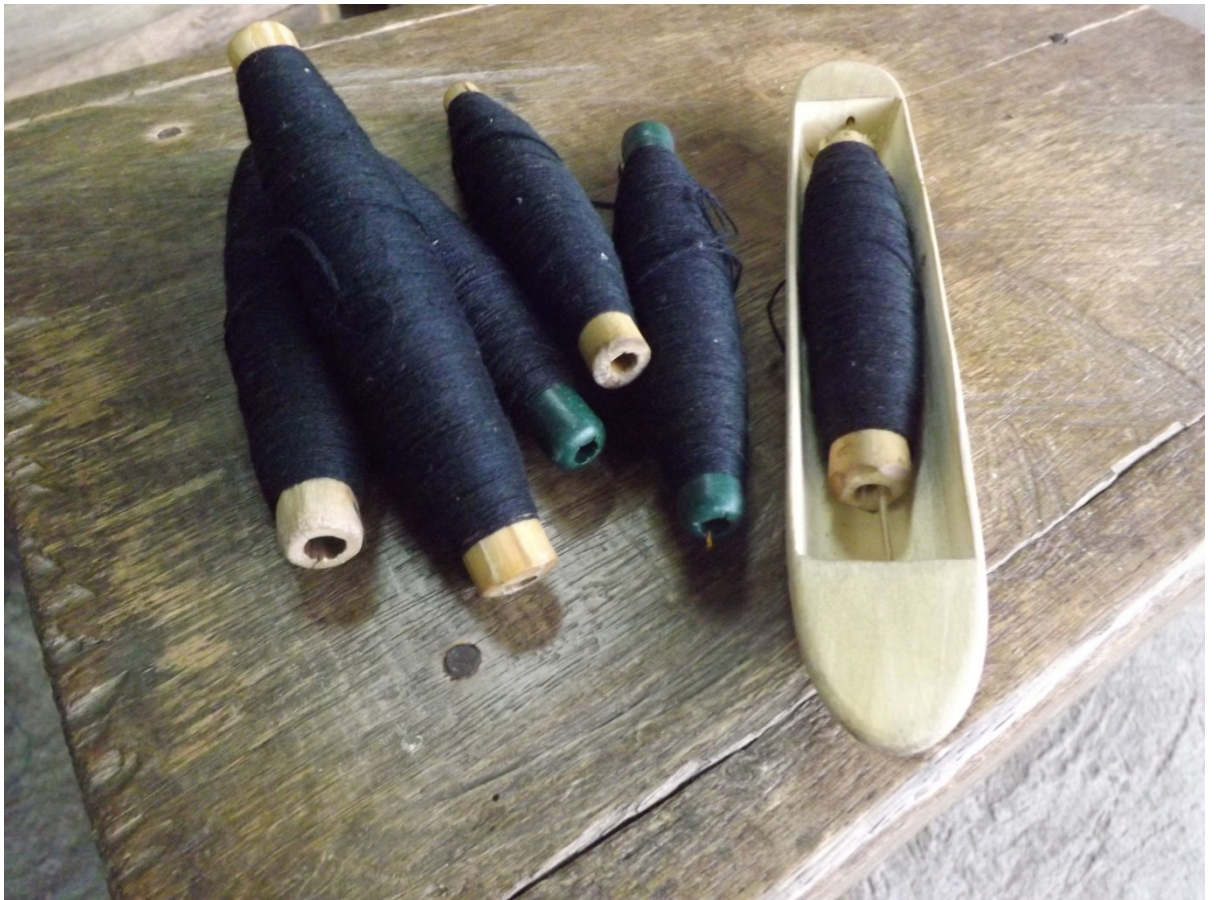
Plate 5- Weft bobbins ready for weaving, October 2012. Photograph by author.
