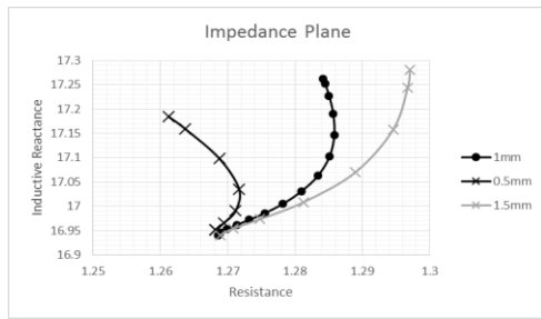
Figure 7: Showing Impedance plane response of internal defects
