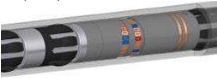
Figure 1 DefHi Eddy Current Probe Configuration
