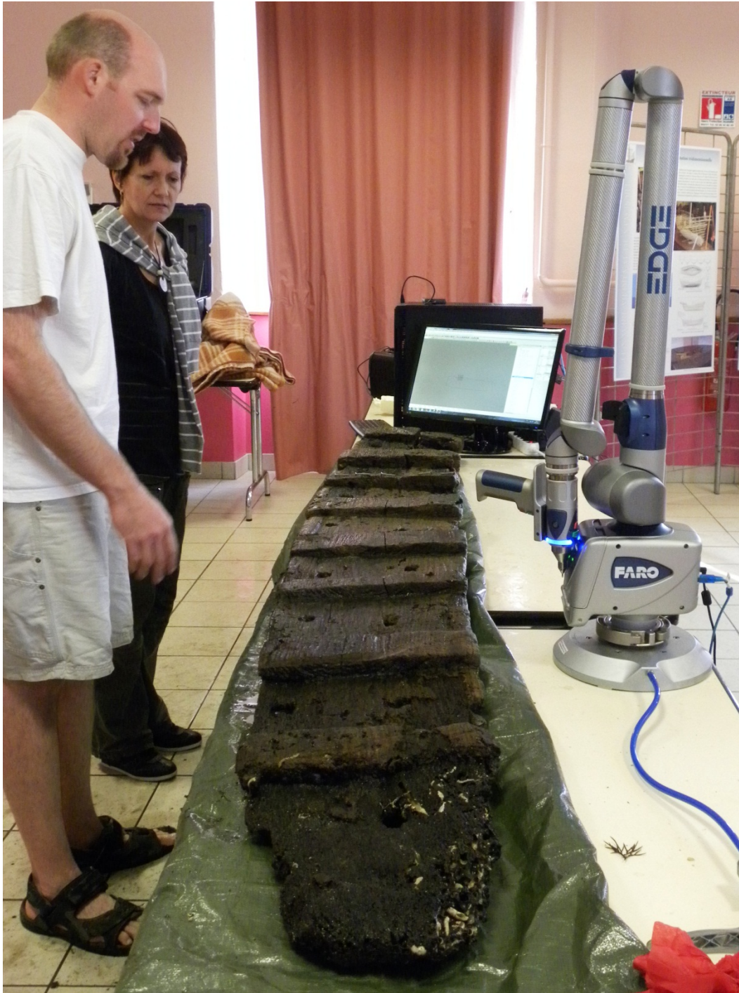
Figure 79. Using a FaroArm contact digitiser to document the outboard face of a stringer recovered from the Aber Wrac'h 1 vessel. Anais Pajot.
