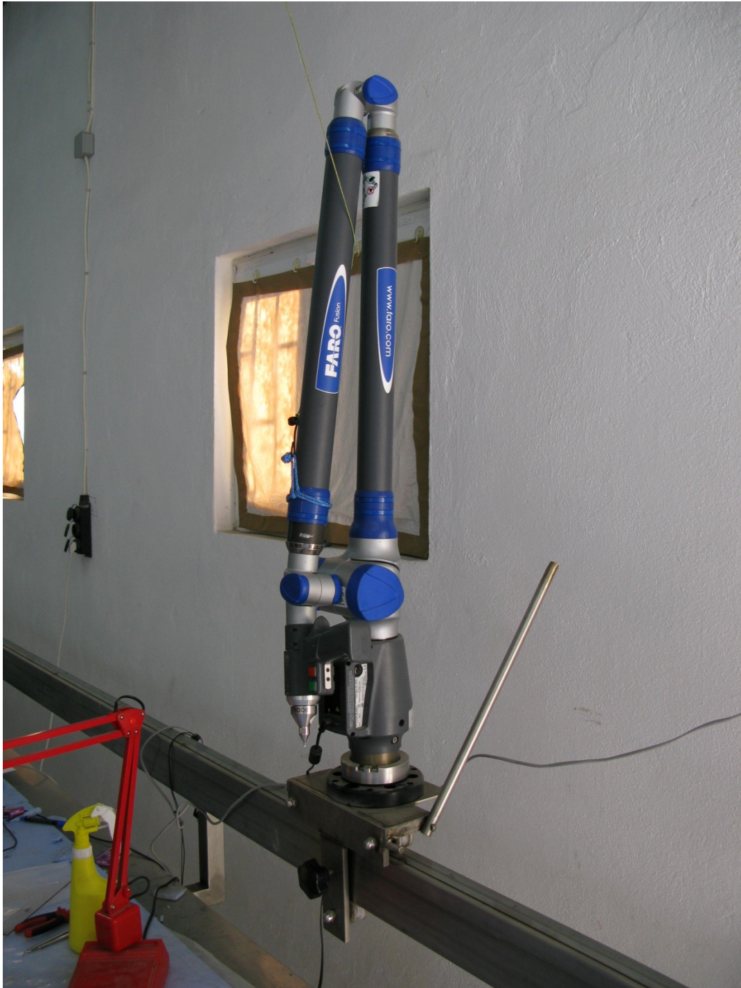
Figure 92. The FaroArm contact digitiser used by the Istanbul University recording team at the Yenikapı excavations. The digitiser was mounted to a rail that ran the entire c.10m length of the recording table. Toby Jones.
