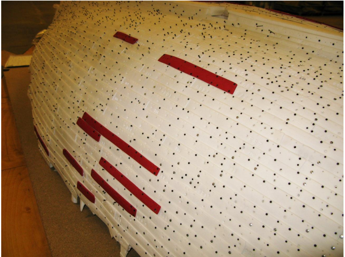
Figure 125. Outboard starboard surface of the inverted model. Note the tangles (patches) modelled in red. Toby Jones.
