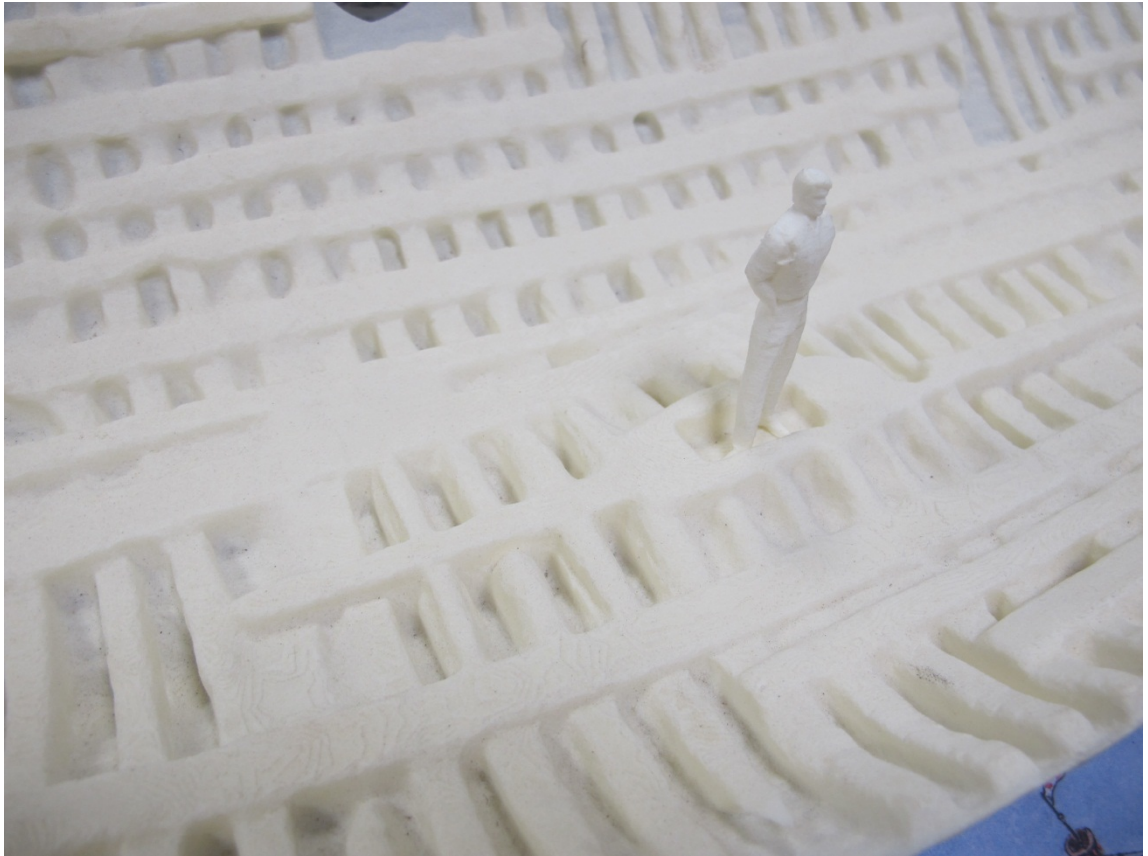
Figure 138. Detail of the 1:30 scale laser-sintered model of the articulated hull remains. Note the removable human figure standing in the mast step rebate. Bow is to the left. Toby Jones.
