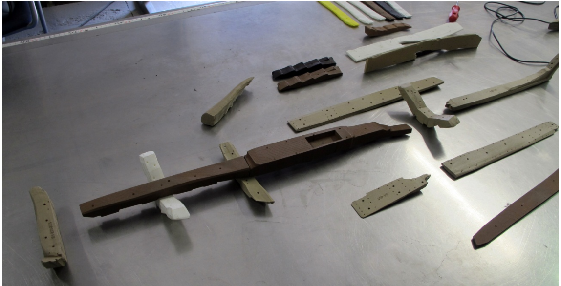
Figure 152. The first batches of additively manufactured scaled model parts from the Doel Kogge project. Toby Jones.
