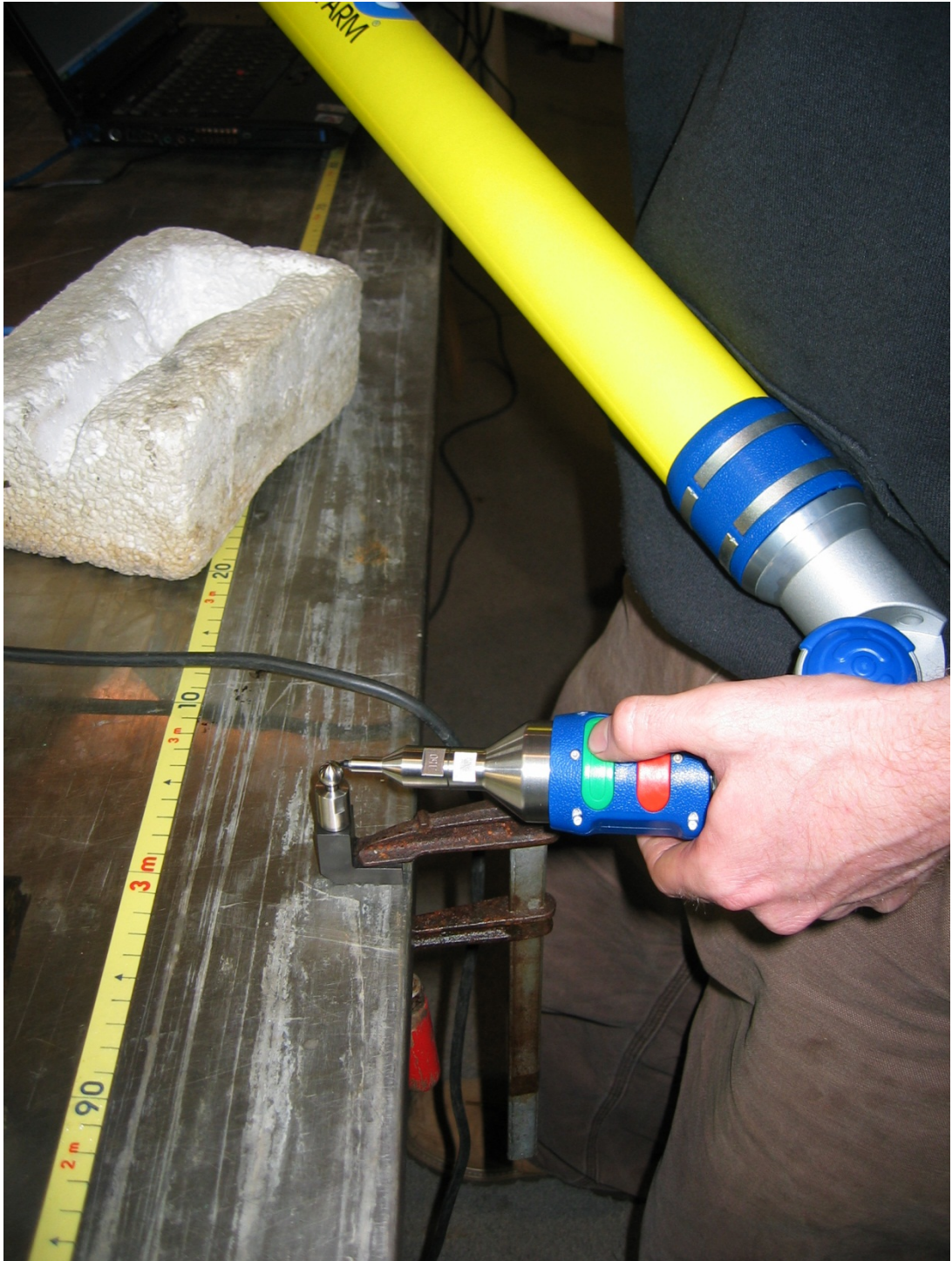
Figure 66. Calibrating the FaroArm contact digitiser. This important check was performed at least once a week, and ensured that the device was in peak operating condition. Toby Jones.
