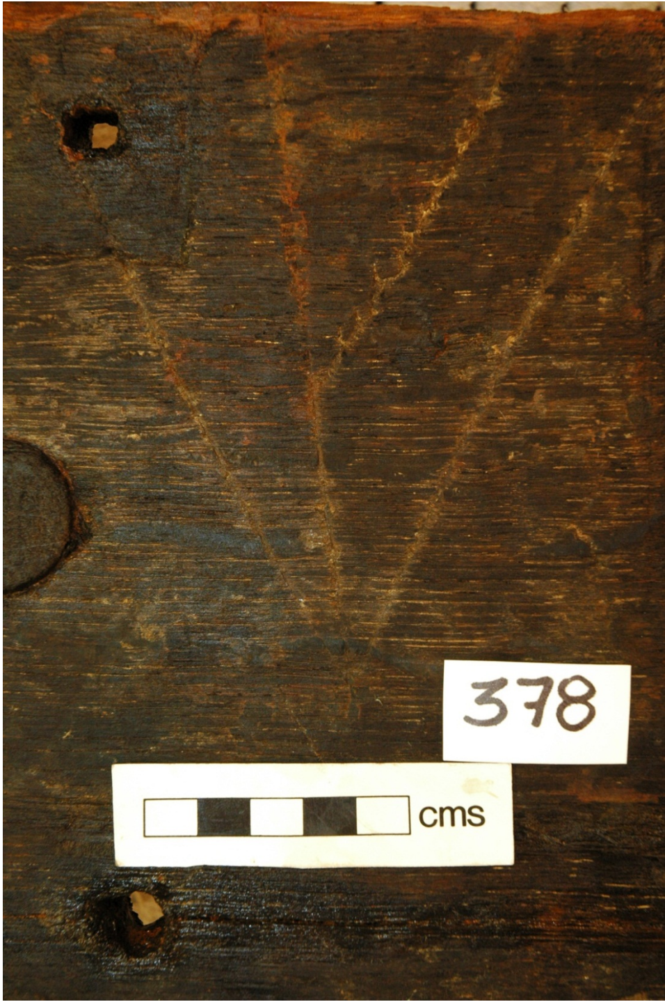
Figure 9. Converging inscribed lines on the inboard face of a hull plank. Note the rove impression in the upper left corner. Newport Museums and Heritage Service.
