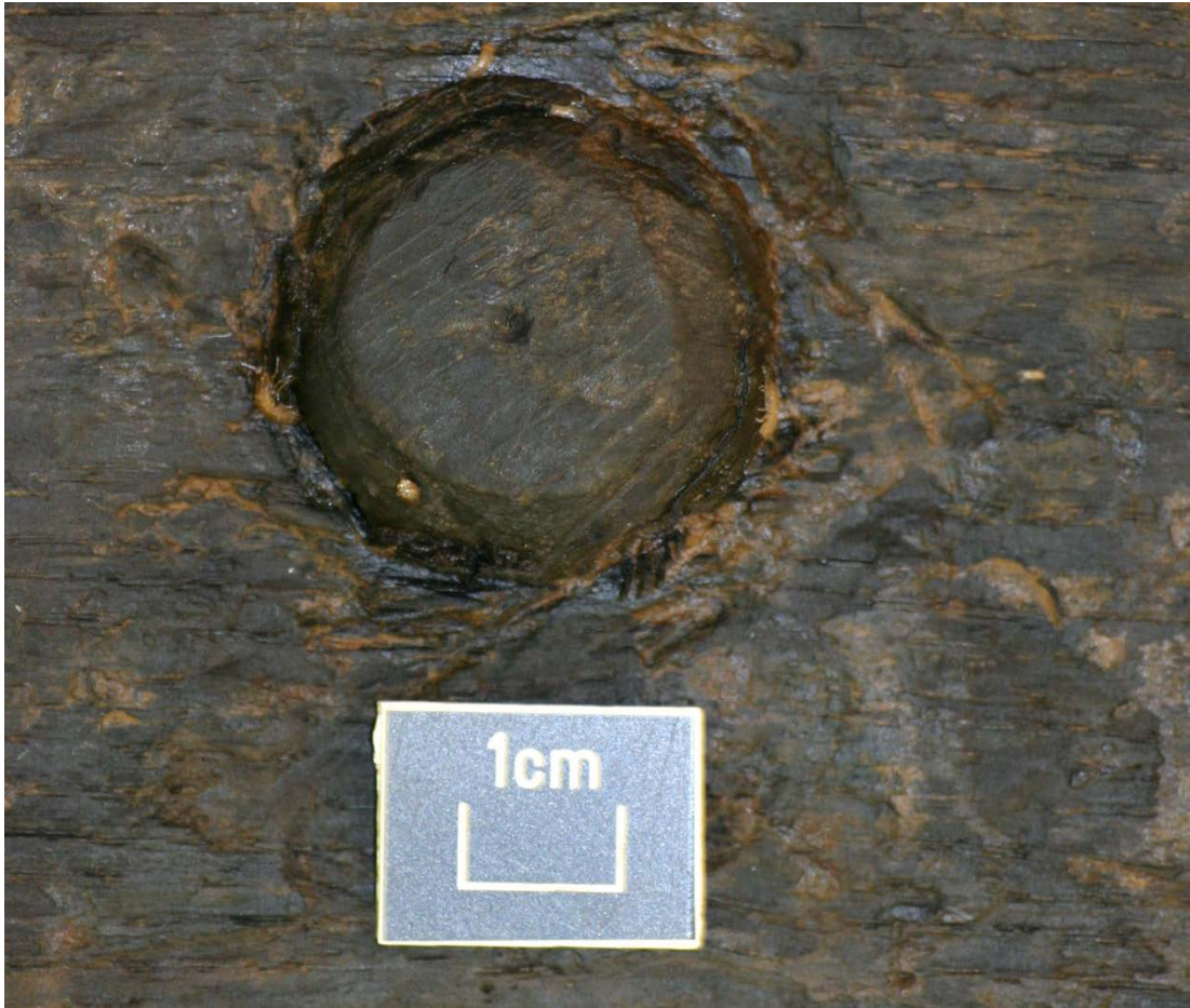
Figure 74. Treenail head on the outboard face of a hull plank. The dimple was created by a lathe during the manufacturing process. Newport Museums and Heritage Service.
