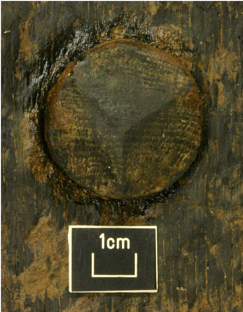
Figure 75. Faceted head of a treenail seen on the outboard face of a hull plank. Newport Museums and Heritage Service.
