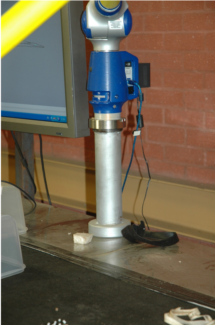
Figure 50. FaroArm Base extension tube. This 300mm long threaded tube increased the range of the contact digitiser considerably. Toby Jones.
