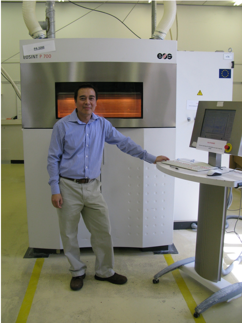
Figure 114. Selective Laser Sintering (SLS) machine at the Manufacturing and Engineering Centre at Cardiff University. The machine was capable of producing several hundred scale model ship parts in each batch. Toby Jones.
