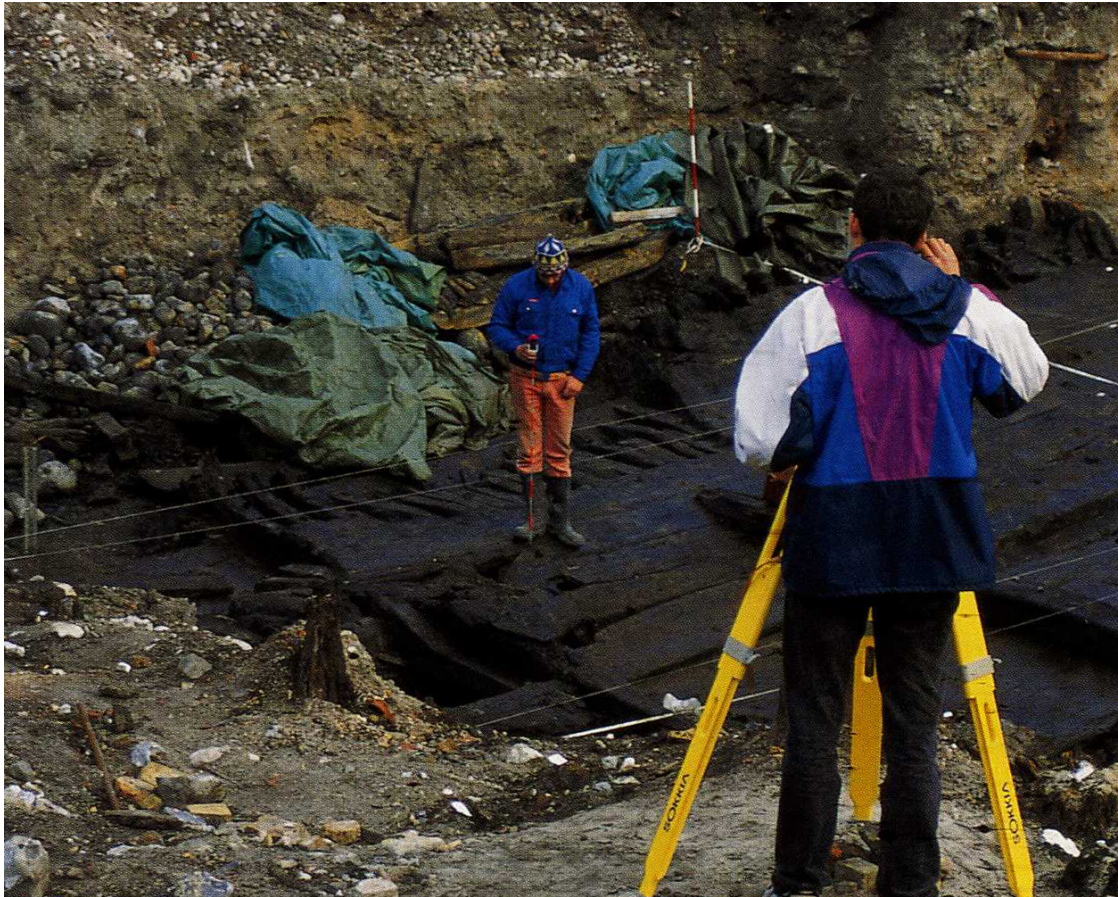
Figure 34. The use of a total station to measure in points on the hull of one of the Renaissance Ships in Copenhagen. After Gyldenkaerne, B., in Lemée, 2006: 83.
