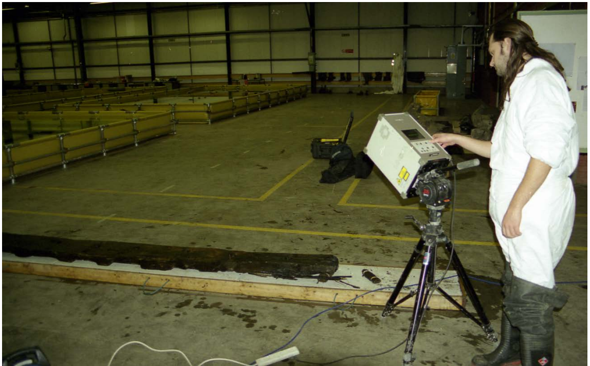
Figure 42. Newport Ship Recording Trials. Using a laser scanner to document a stringer. Newport Museums and Heritage Service.
