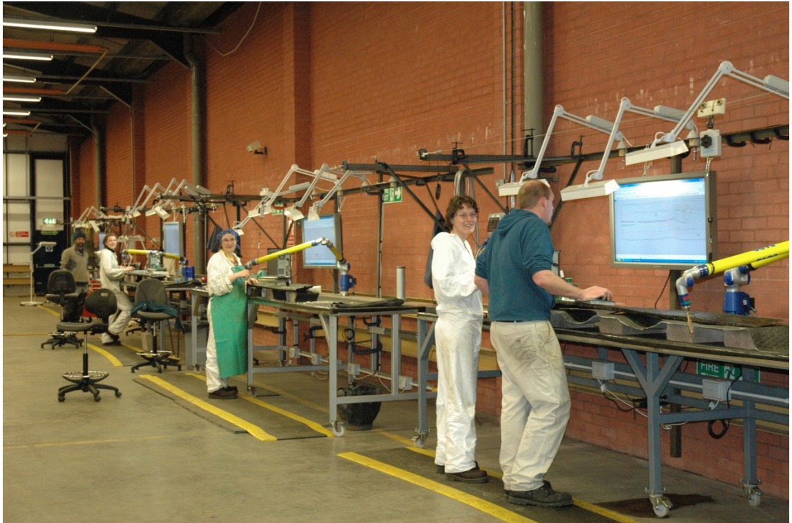
Figure 46. Four identical contact digitiser work stations were created to efficiently record the large assemblage. Newport Museums and Heritage Service.
