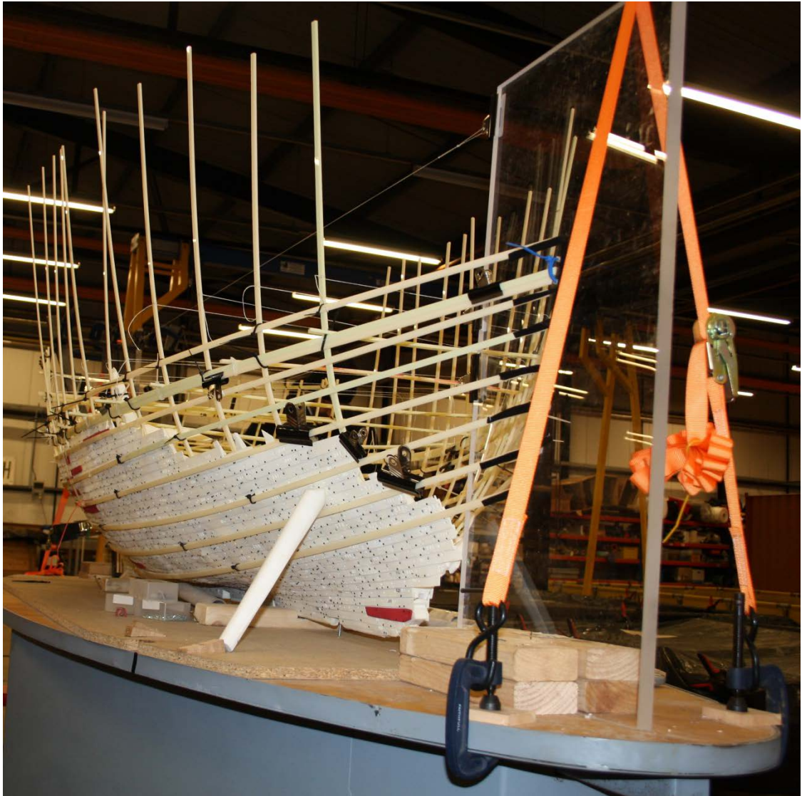
Figure 148. The physical scaled model was firmly attached to the modelling table and the starboard twist in the bow and stern was largely removed by using clamps, screws and braces to force the physical model into a more correct shape. Toby Jones.
