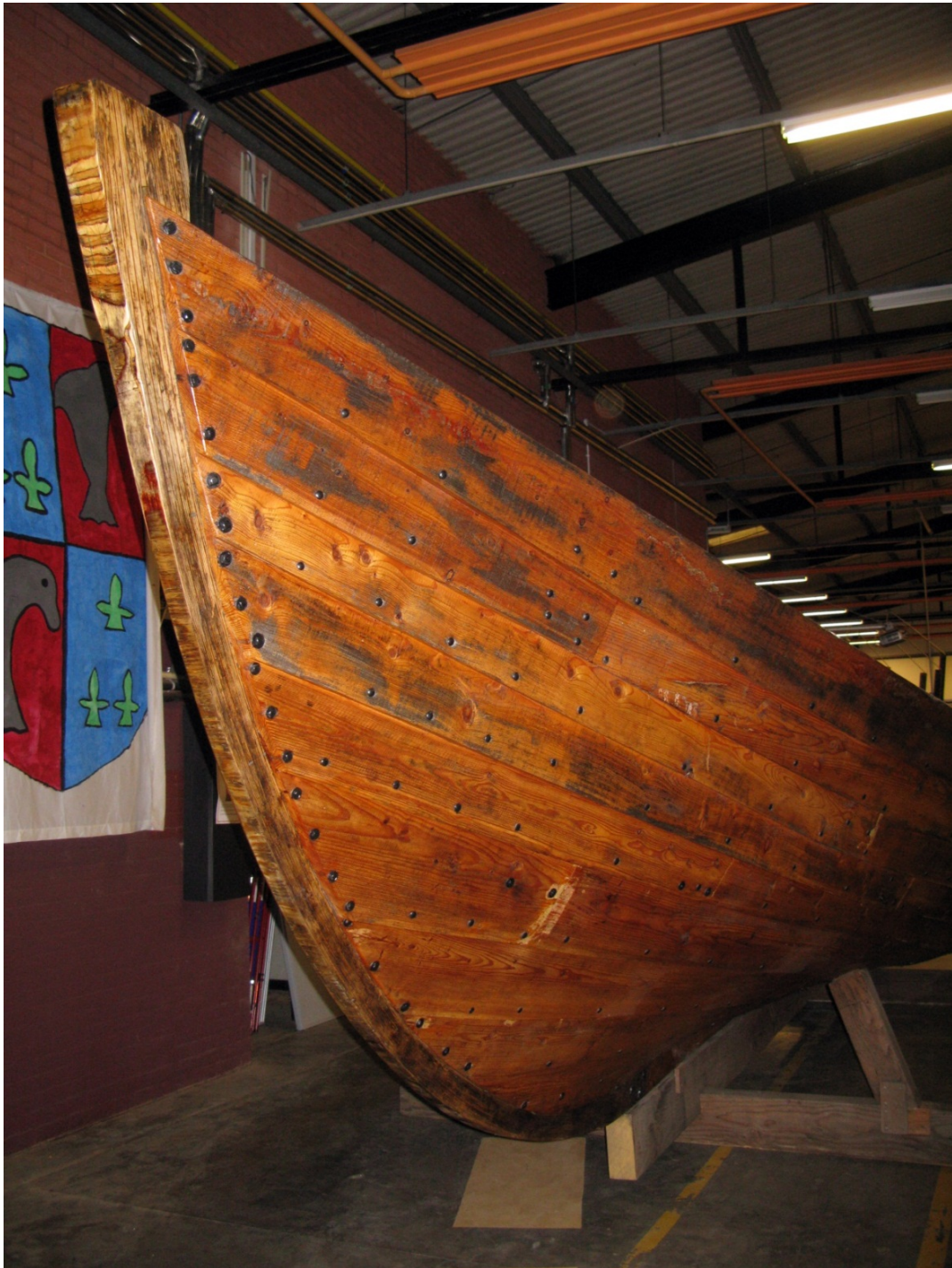
Figure 32. A partial 1:1 scale model of the Magor Pill vessel. Toby Jones.
