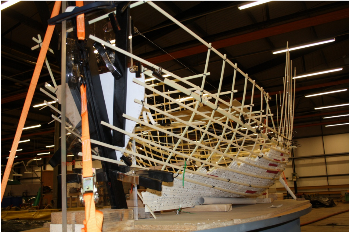
Figure 147. The transom stern fitted to the physical scaled model. Toby Jones.
