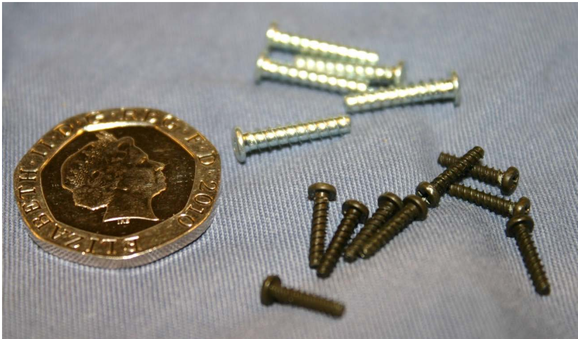
Figure 127. Threaded micro-fasteners used to assemble the hull form model. The smaller black screws were used in clenched nail holes, while the larger silver screws were used in treenail holes. Toby Jones.
