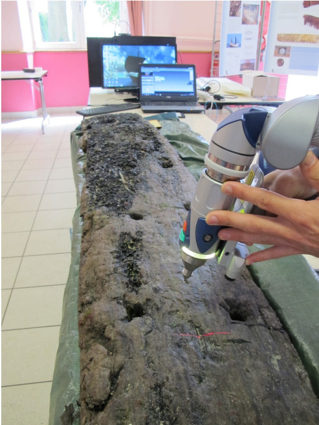
Figure 77. Using a FaroArm contact digitiser and associated laser scanner to document a stringer from the Aber Wrac'h 1 vessel. The emitted laser from the scanner can be seen as a red stripe in the foreground. Anais Pajot.
