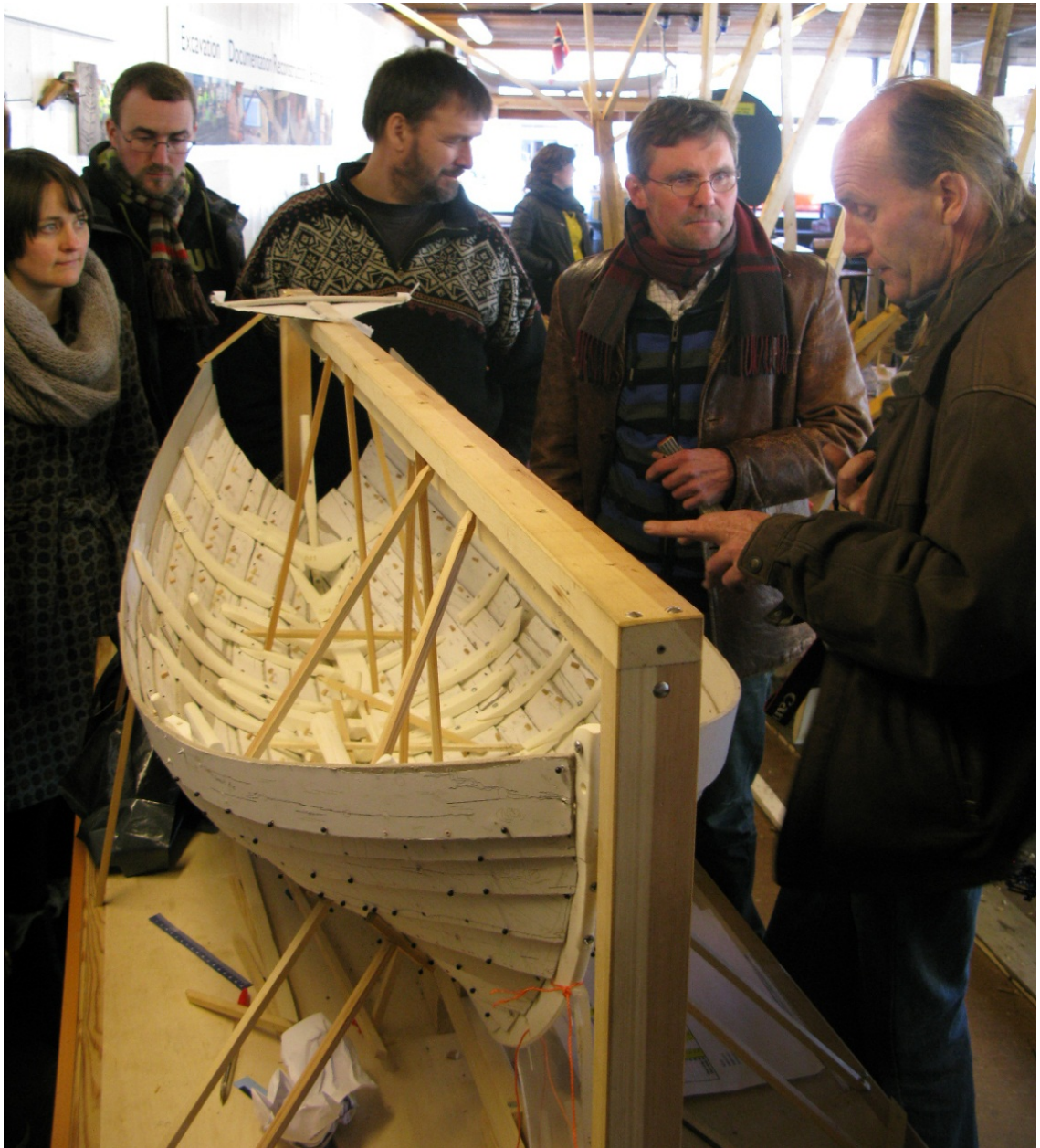
Figure 151. Composite scaled physical hull form model of the late 16th century Barcode 6 shipwreck at the Norwegian Maritime Museum. The 1:5 scale model was created using a combination of laser sintered framing and hand-cut cardboard planks. The same methodological processes used on the Barcode 6 shipwreck were used to record and model the Sjørenga 7 vessel. Toby Jones.
