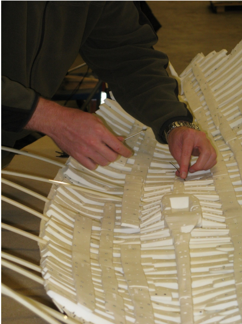
Figure 140. Transverse ribbands were threaded through the inter frame spaces, under the stringers (and keelson in amidships area), near every fifth frame station. Newport Museums and Heritage Service.
