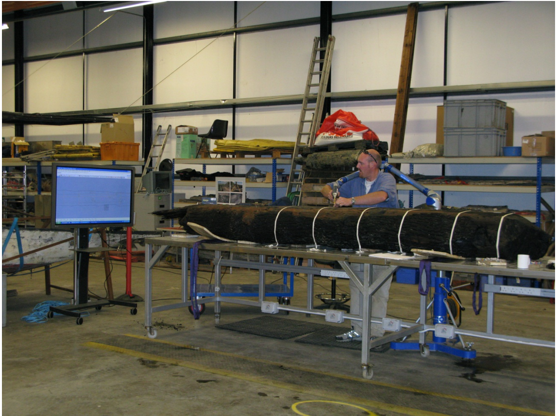
Figure 49. Archaeologist using a contact digitiser to record one of the large struts found under the Newport Ship. The use of tripods and moveable support tables and computer monitors allowed for flexible approaches to setting up the workspace. Newport Museums and Heritage Service.
