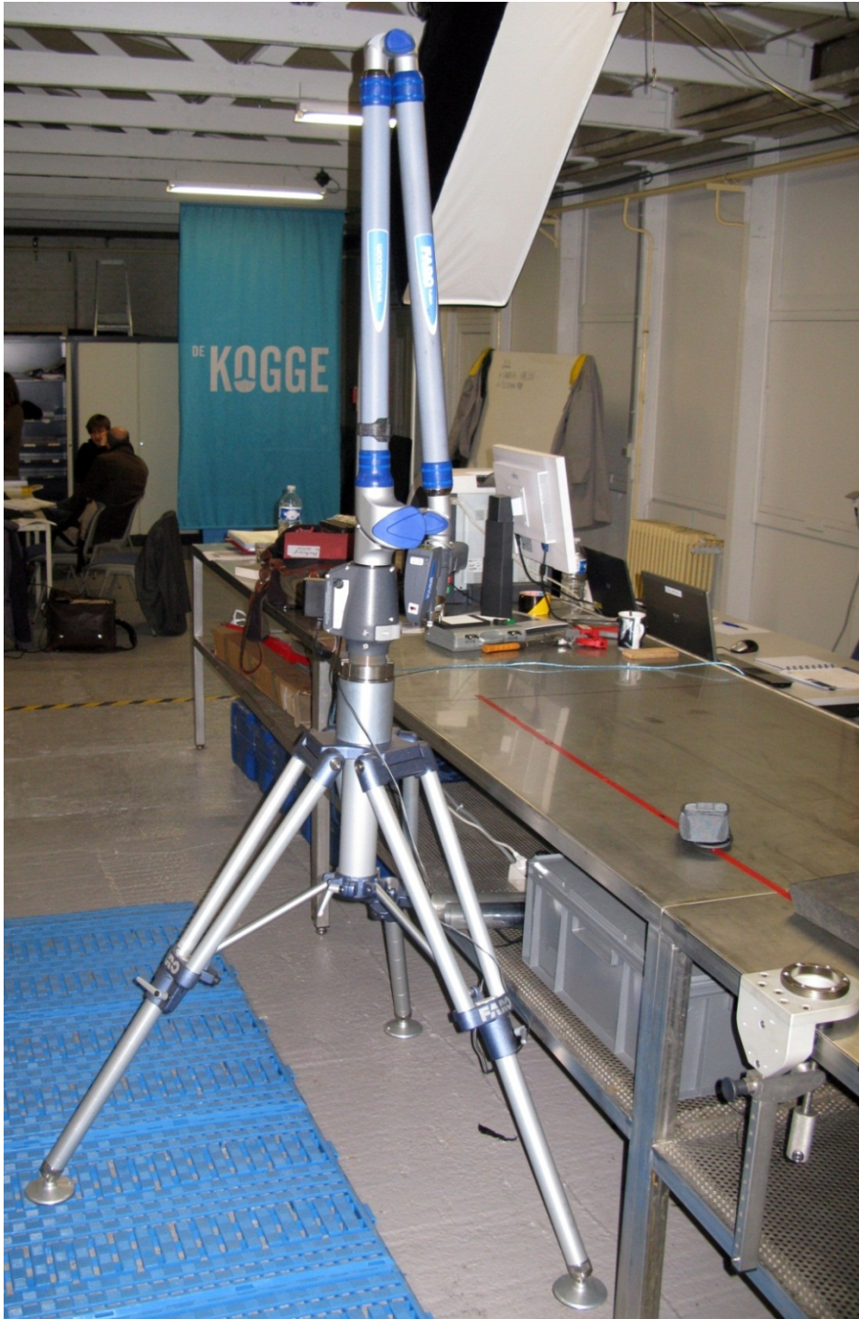
Figure 88. The recording tables and contact digitiser arrangement used at the Doel Kogge Project in Antwerp, Belgium. Note the moveable clamp with mounting ring in the lower right. Toby Jones.
