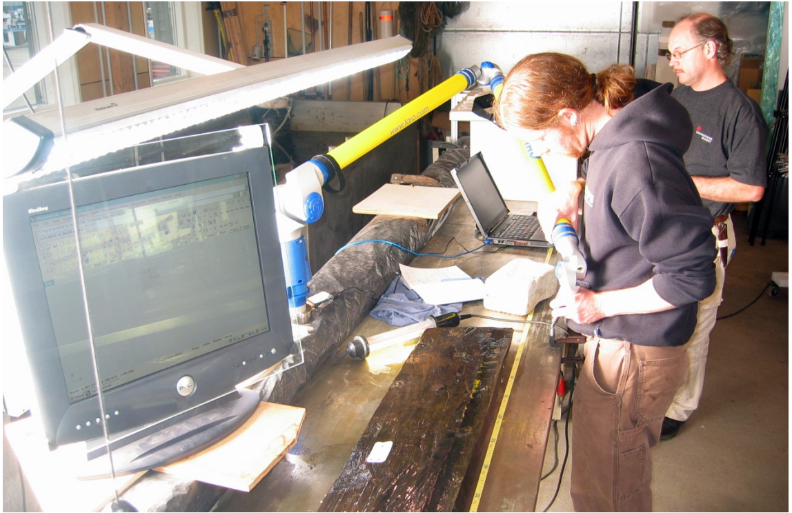
Figure 36. Documenting a ship's timber using a contact digitiser at the Viking Ship Museum in Roskilde, Denmark in 2004. Toby Jones.
