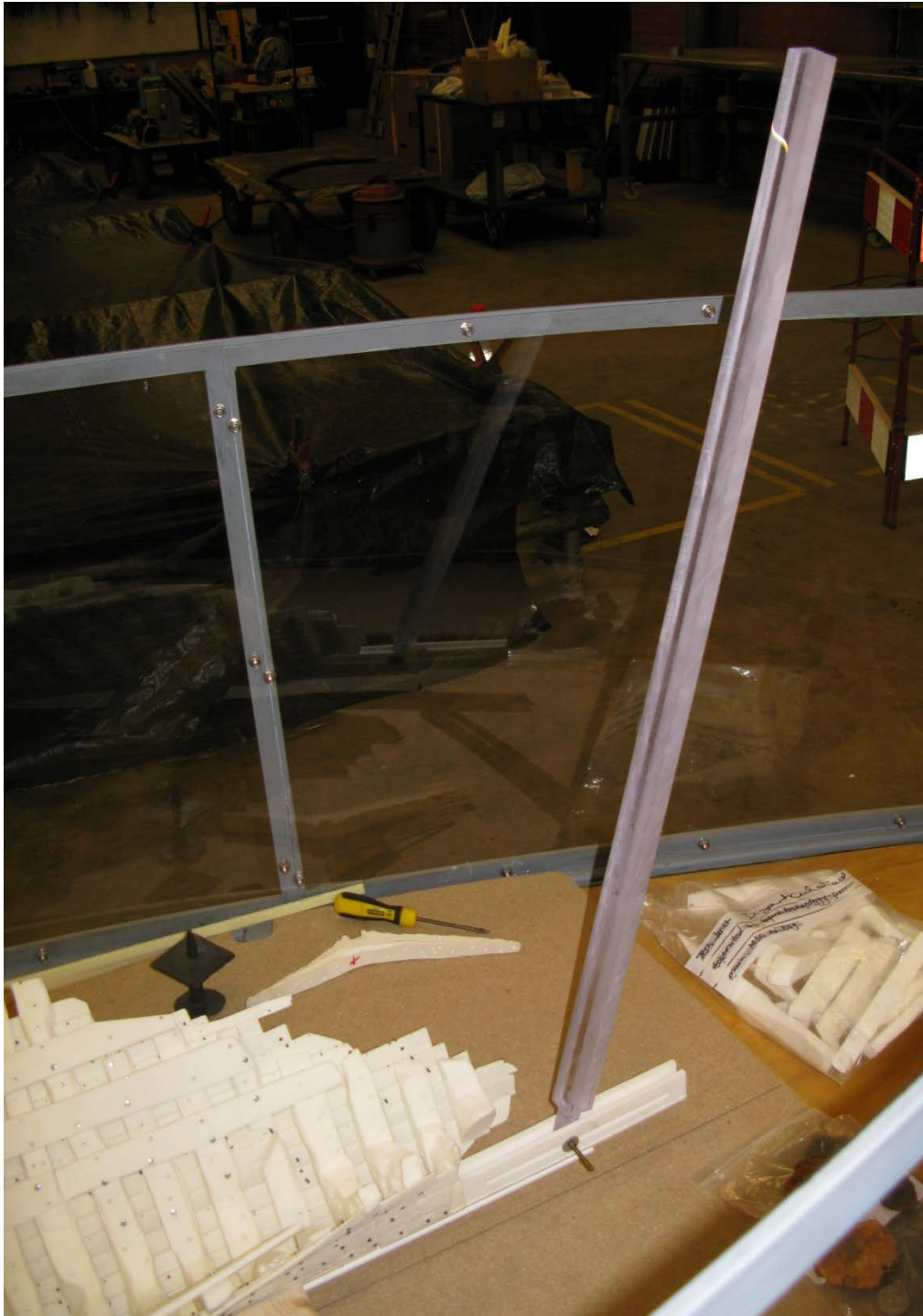
Figure 144. The second attempt to create a suitable adjustable stern post. Toby Jones.
