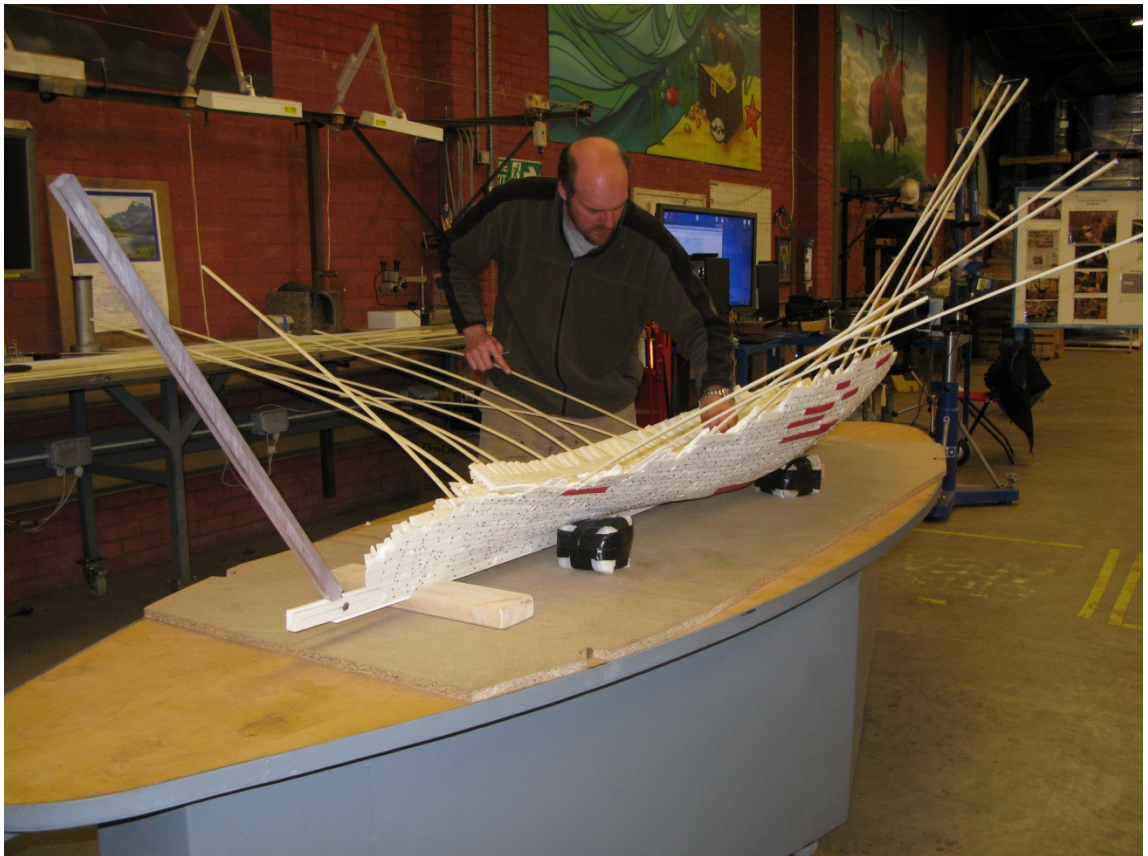
Figure 139. Author fitting plastic transverse ribbands to the model. Newport Museums and Heritage Service.
