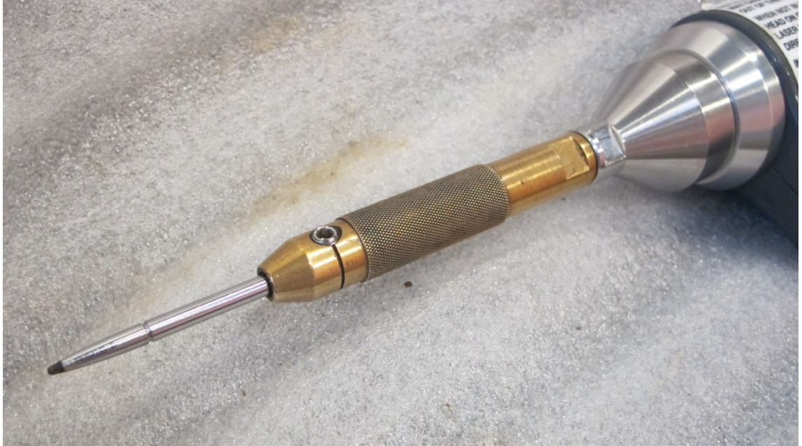
Figure 57. Machined FaroArm contact digitiser probe tip holder with a non-marking PDA stylus used as a probe tip. Toby Jones.
