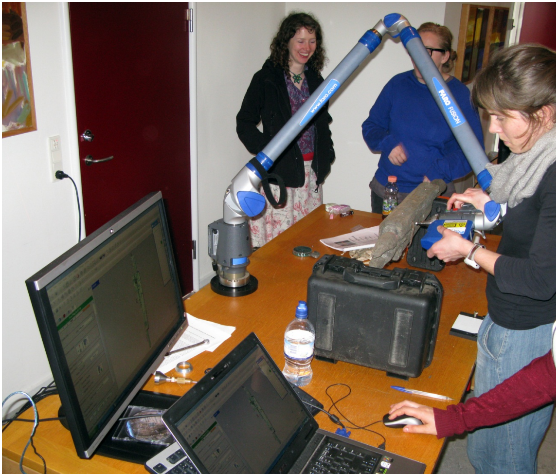
Figure 87. Students at the University of Southern Denmark learning how to use the contact digitiser, associated laser scanner and relevant software. Toby Jones.
