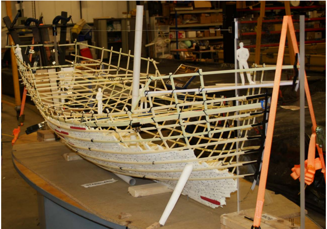
Figure 150. The completed 1:10 scale physical hull form model of the Newport Medieval Ship with ribbands ghosting-in the missing areas of the hull. Toby Jones.
