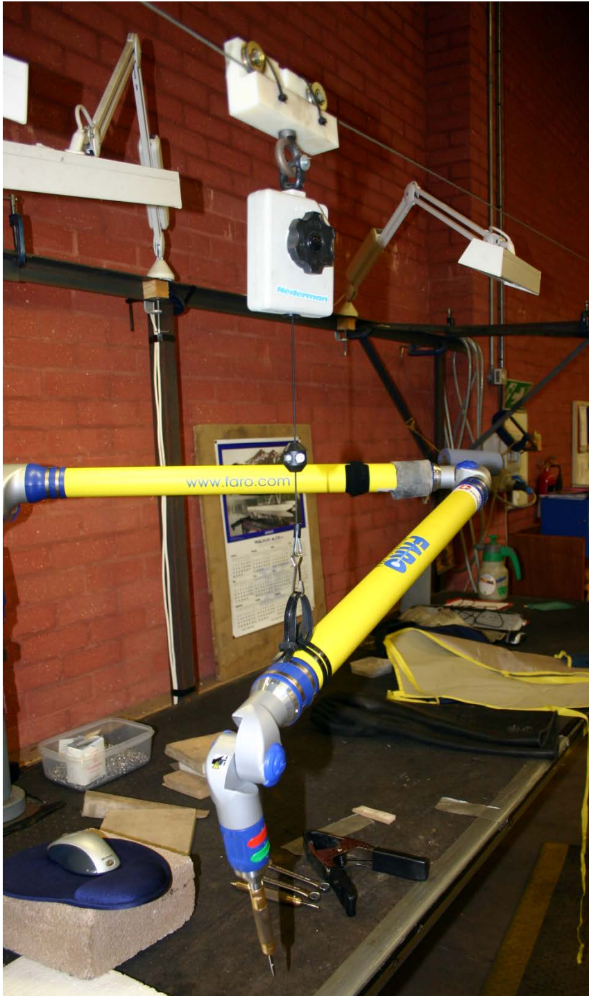
Figure 51. Contact digitiser supported by a counterbalance system suspended from a carriage and cable. Toby Jones.
