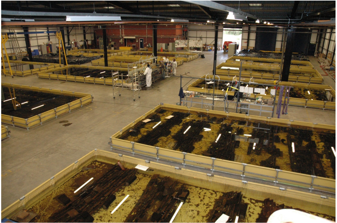
Figure 45. The Newport Medieval Ship Centre. Timbers were organised by function (planks, framing timbers, stringers, etc. and placed in tanks for storage. Note the mobile overhead gantry, used to handle larger timbers, in the top left. Toby Jones.
