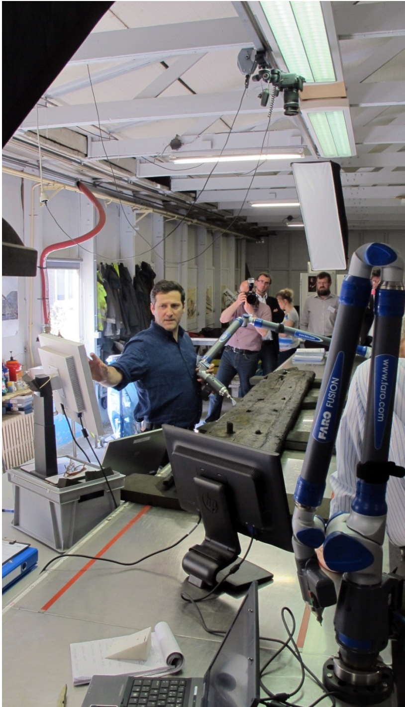
Figure 89. Archaeologist at the Doel Kogge Project using a FaroArm contact digitiser to document a ship's timber. Note the overhead framework and associated photographic equipment and light sources. Toby Jones.
