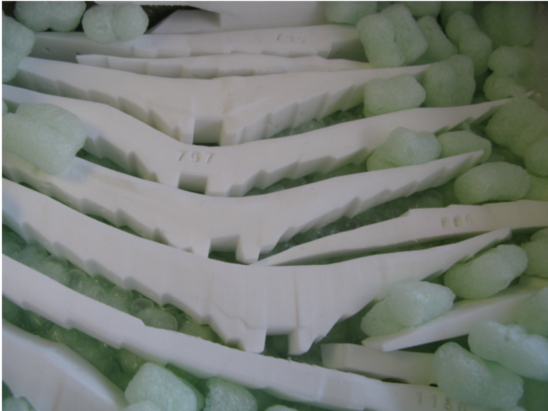
Figure 119. Completed framing timber scale model pieces. Digital solid models of each timber were emailed to the Manufacturing and Engineering Centre at Cardiff University. The finished physical model pieces from each batch were packaged and then posted back to the ship centre. Toby Jones.
