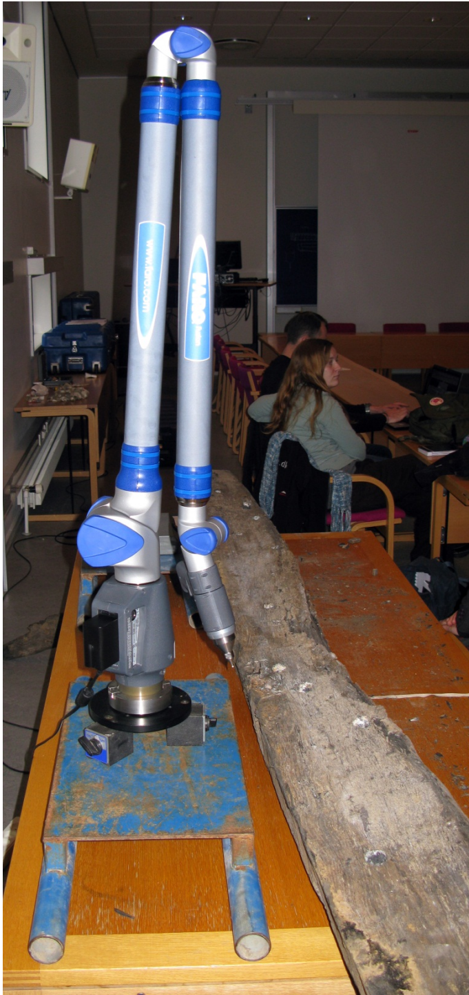
Figure 41. A FaroArm contact digitiser magnetically clamped to a portable heavy steel base. Toby Jones.
