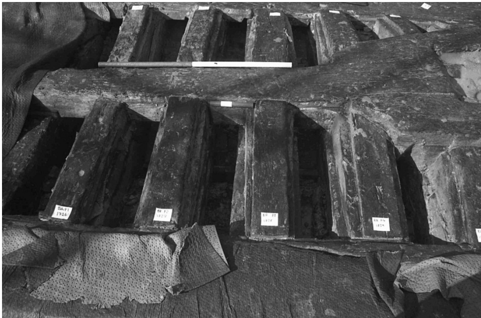
Figure 131. Detail of the in situ mast step/keelson and forward-most braces. Compare to Figure 130. Bow is to the left. Newport Museums and Heritage Service.
