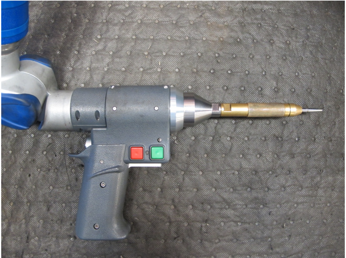
Figure 56. The pistol-grip handle and custom made probe tip holder of the FaroArm contact digitiser. Toby Jones.
