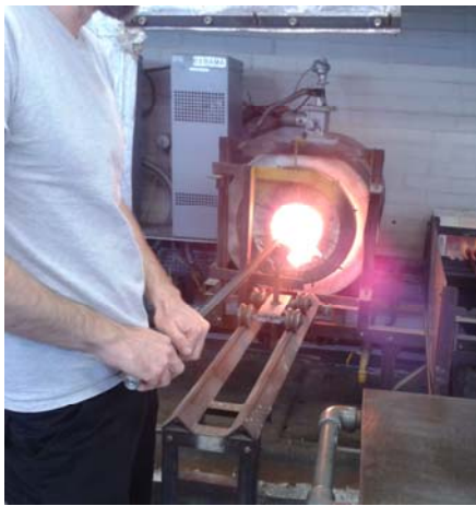
Figure 16. Heating in glory hole
