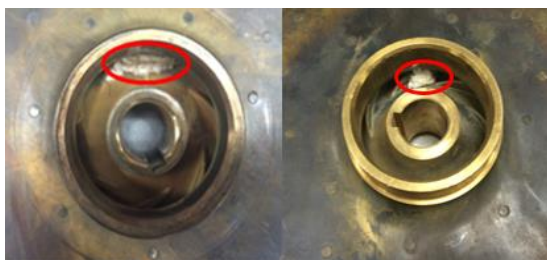
Figure 1 2 The impeller inlet blockages
