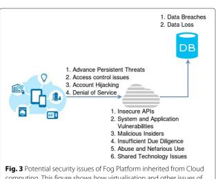
computing. This figure shows how virtualisation and other issues of Cloud platform can effect Fog platform as well
