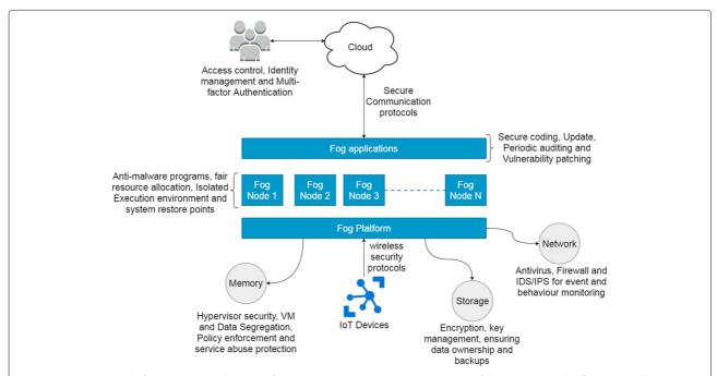
**Fig. 4** Fog Computing Platform and the deployment of security solutions on various components of the Fog system. This figure shows how and where proposed security solutions can be placed and help in eliminating various security flaws
