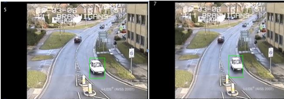
(a) Algorithm1: Foreground detection and blob analysis (b) Algorithm2: Optical Flow and Blob analysis Figure 12. Test 2, frames from both algorithms FDBA and OFBA after tracking.
