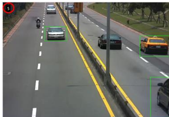
Figure 8. Algorithm2-OFBA: Frame with tracking and counting of vehicles.
