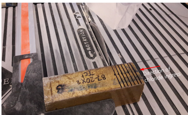
Figure 2. Cutting of mortar slices for chloride profile analysis
