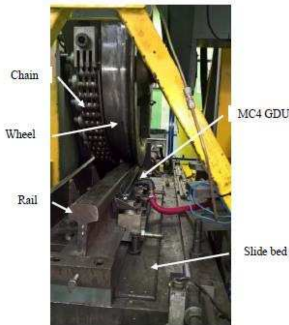
Figure 5- Set-up of MC4-GDU on FSR
