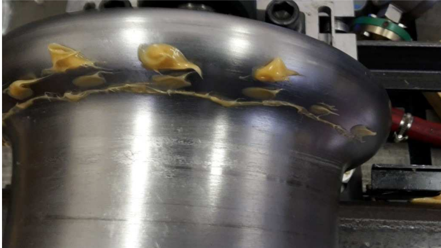
Figure 13- Pick up of grease onto wheel from one pass through the standard MC4 applicator
