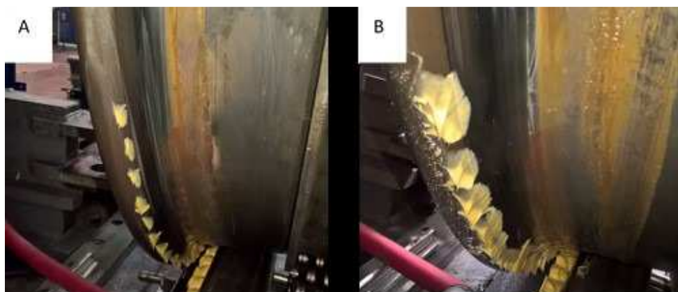
Figure 21- Pick-up of grease onto wheel from one wheel pass at lateral displacement 6.5mm using A) standard MC4 GDU, B) MC4-GG
