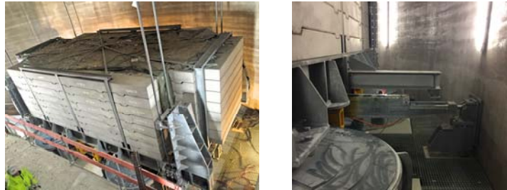
Fig. 2. Left: Pendulum rope supported TMD mass – Right: Linear Motor as actuator
