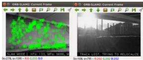
Figure 3: Two frames from ORB-SLAM that results in the map shown in Figure 4. ORB features are marked as green squares in the left hand image. In the right hand image no features appear since tracking has been lost due to a sudden change in lighting conditions.
