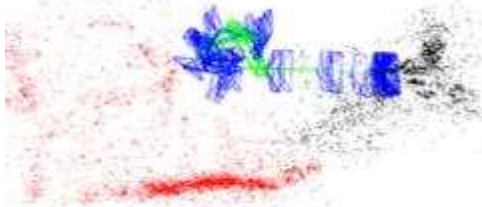
Figure 4: The map produced by ORB-SLAM. The key frame locations can be seen by the blue rectangles, the current keyframe as a green rectangle and the progression of the robot also in green. The red map points show the local visible map.
