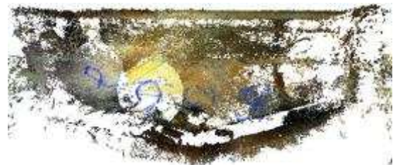
Figure 5: The SfM reconstruction completed using Zephyr Aerial SfM software. The same dataset used for ORB-SLAM was used for the reconstruction. The camera positions can also be seen as blue triangles.
