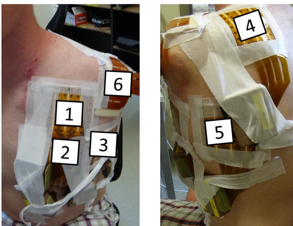
Figure 2. Matrix constellation for Session 4 (Session 5 was as similar as possible), with four high-density 8 x 8 electrode matrices on the chest (left) and two on the back (right), covering the six reinnervated spots used for prosthesis control.
