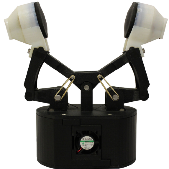
Fig. 1. The GR2 gripper with integrated TacTip sensors.
