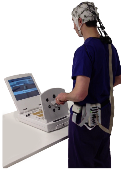
Figure 1: A participant wearing the mobile EEG cap. Data recorded at each electrode is transferred wirelessly to the amplifier connected to a standard PC. The participant is performing the MISKT task in a laparoscopic box trainer.
