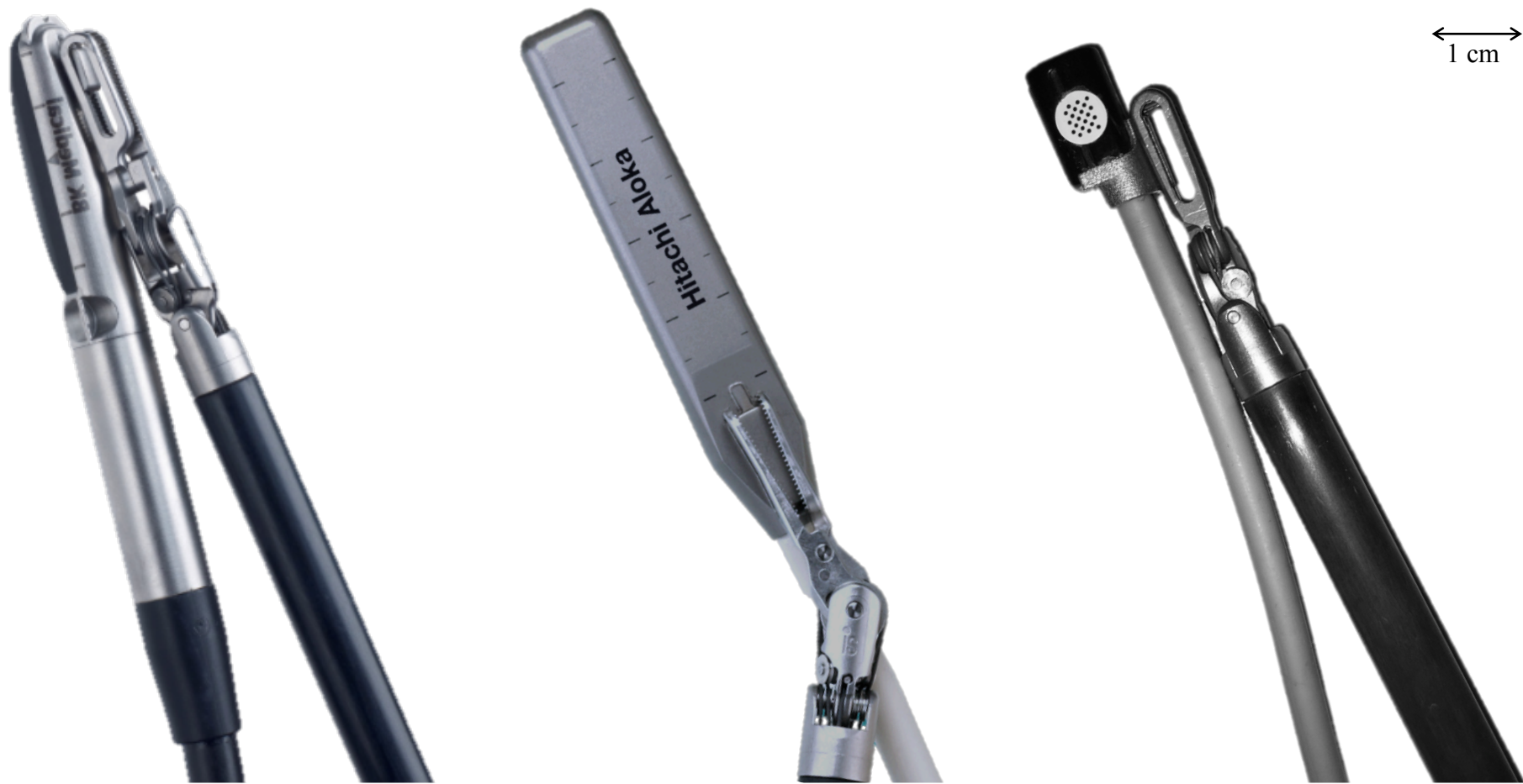
Figure 8.1.1 – Commercially available robotic ‘drop-in’ ultrasound probes (left to right: BK medical ProART™ and Hitachi Aloka UST-5550-R) alongside the research platform setup of a Aloka Hitachi Aloka UST-533 probe with imperial designed ultrasound clip.
