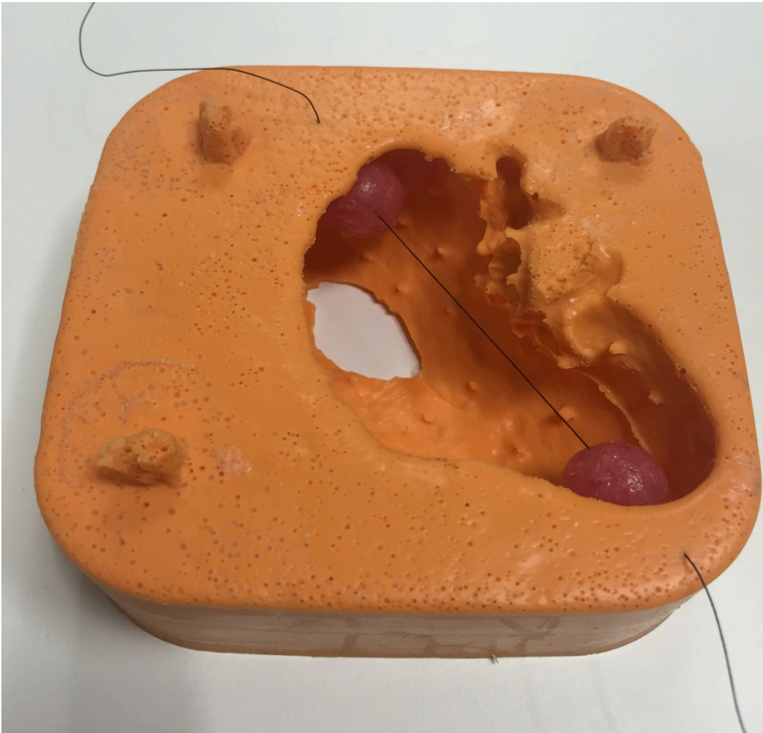
Figure A3.3.2 – Tumour phantoms in place prior to filling of renal mould
