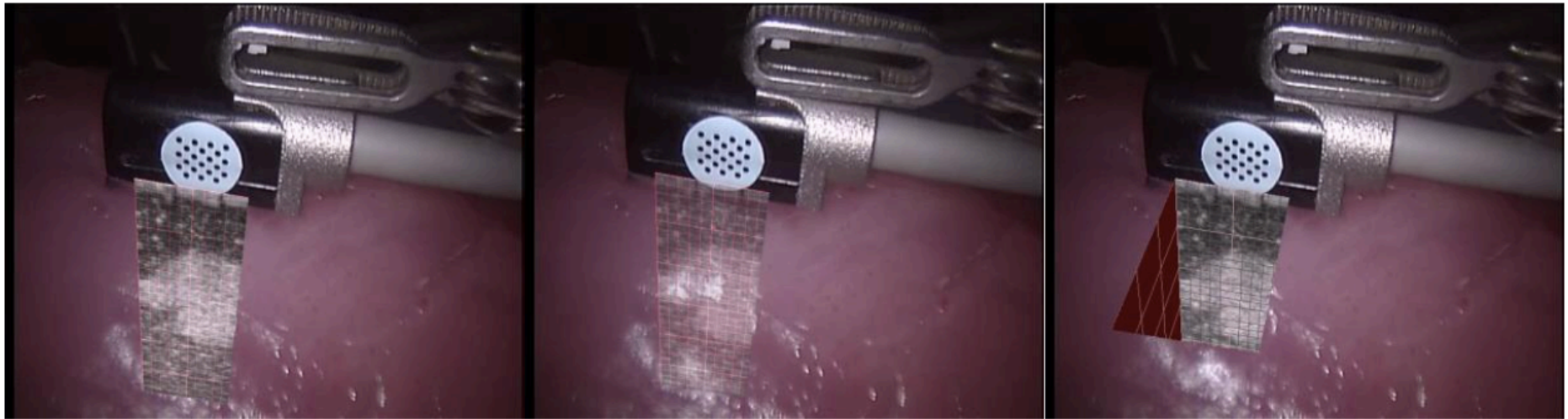
Figure 8.1.7 – The different modes of image display available to the surgeon. From left to right: Solid overlay, transparent overlay and cutaway view, all displays included a 1mm ruler. The modes are demonstrated on a PVA cryogel phantom (See Appendix 4)
