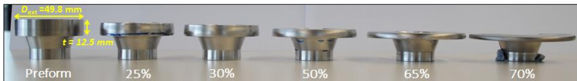
Figure 3. Sequence of rotary forged flanged-test pieces with increasing thickness reduction
