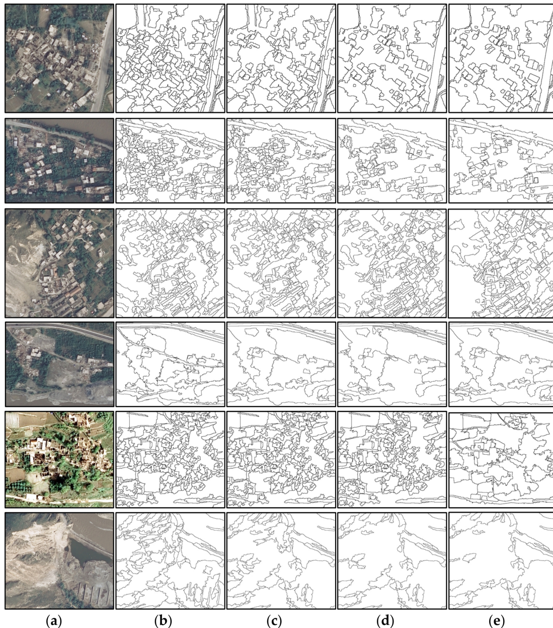
Figure 5. The ground truths of six test images interpreted by different experts. (a) Original images: from top to down are T1–T6; (b–e) Four expert interpreted ground truths.
