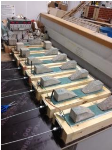
Figure 2 Accelerated corrosion of tendons via power supply (top left)
