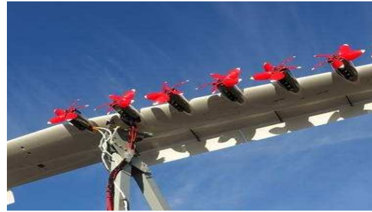
Figure 18. NASA LEAPtech wing during tests (NASA Web site).
