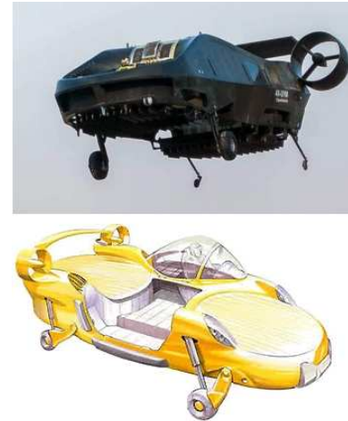
Figure 32. Xplorair AirMule prototype and XHawk drawing
