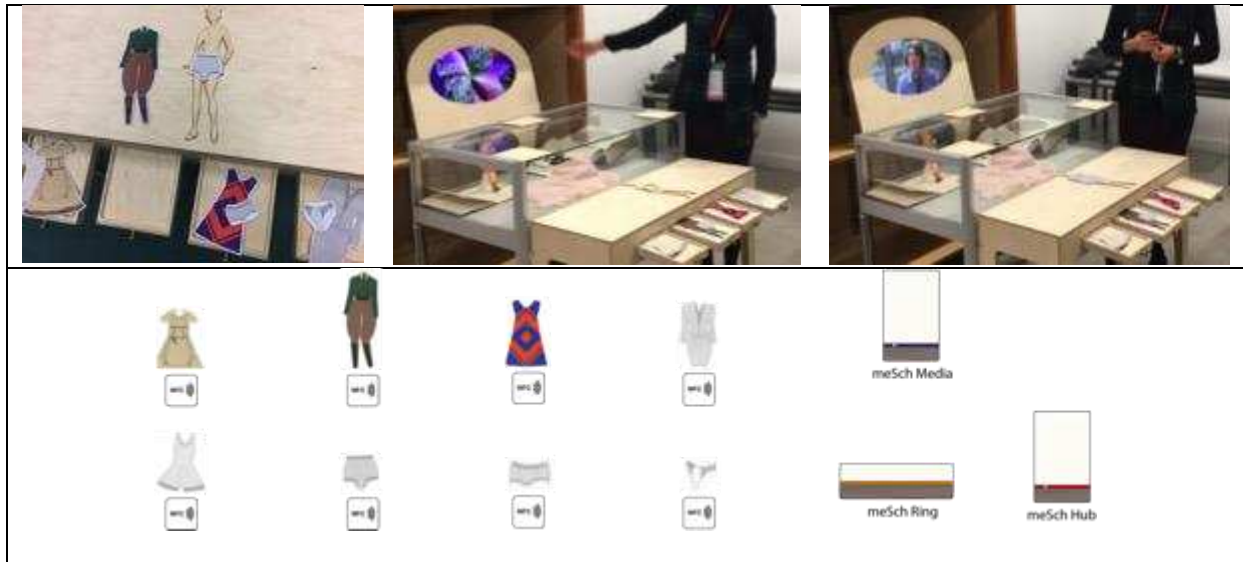
Figure 4. (top) Four drawers on the vanity desk hold different decades (20s, 40s, 60s, 80s) and contain personal stories (underwear) and social changes (dresses) that, when placed on the mannequin play different videos (the 80s in the pictures). (bottom) Each cut-out has a NFC tag, a Ring is under the mannequin and a Media node connects to the screen.
