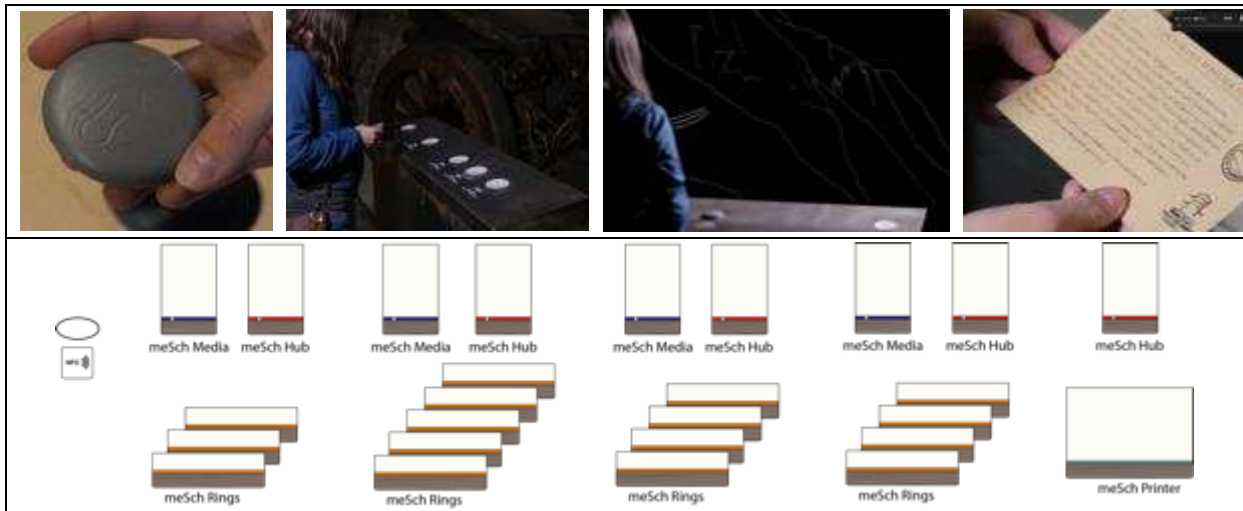
Figure 5. Voices from the Past in Fort Pozzachchio is a permanent installation. (top) At the entrance the visitor receives a pebble used to activate content at different station along the visit; when leaving the visitor returns the pebble to the desk and receives a personalised postcard with a summary of their visit. The pebble has an NFC read-write; each station has a set of Rings, one for each personal story, a Hub that controls the Ring and a Media node to project the content. At the exit another Hub controls the printing of the personalised postcard. The many Hubs are needed here as there is no WI-FI signal due to the harsh environment: a bomb shelter dug into the mountain.
