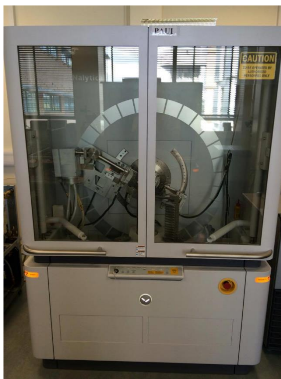
Figure 3.3. Panalytical Empyrean diffractometer in Bragg-Bretano geometry with a Ge (220) monochromator and Cu K\alpha_1 radiation ( \lambda=1.5406 \text{ \AA} )
