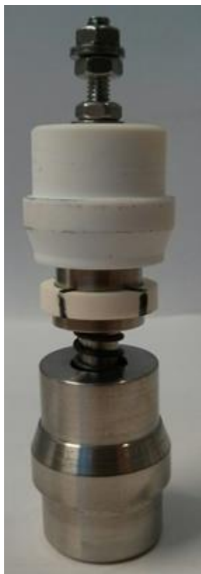
Figure 3.12. Internal parts of “Swagelok” cell for electrochemical measurements
