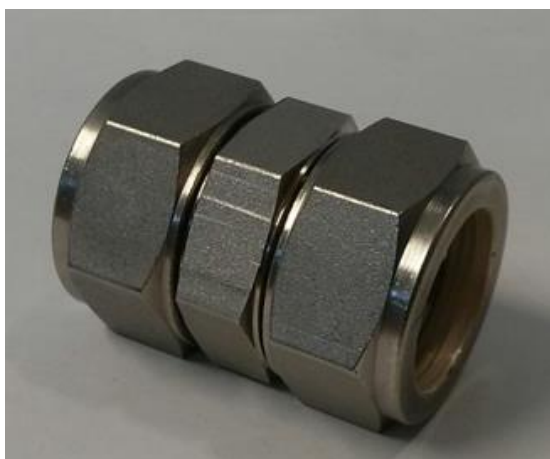
Figure 3.11. External part of “Swagelok” cell for electrochemical measurements
