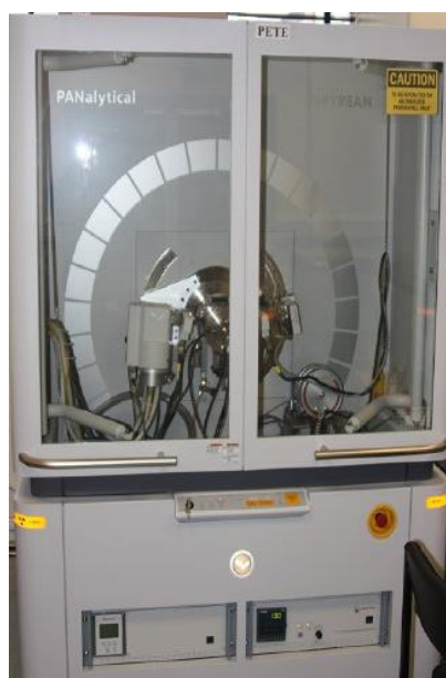
Figure 3.4. Panalytical Empyrean diffractometer with Mo\ K\alpha_{1,2} radiation, \beta -filter and an X'celerator RTMS detector, equipped with an Anton Paar HTK1200N furnace
