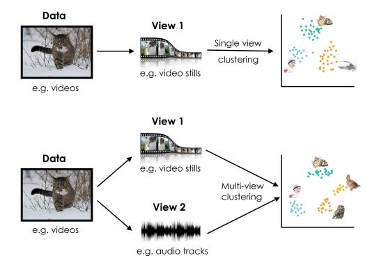
Figure 4.3: Schematic of (top) single-view and (bottom) multi-view clustering. Multi-view clustering techniques can produce different clustering solutions to single-view methods applied to the same data set.
