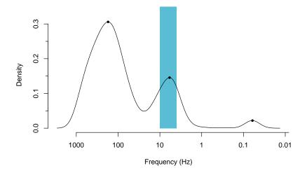
Figure 3.1: Detection of theta bursting on an electrode. Plot shows the smoothed log-adjusted ISI histogram from an electrode with peaks marked. Blue box shows the frequency region representing theta bursting. An electrode was classified as theta bursting if one of the peaks falls within this region. Figure adapted from Charlesworth et al. (2015).
