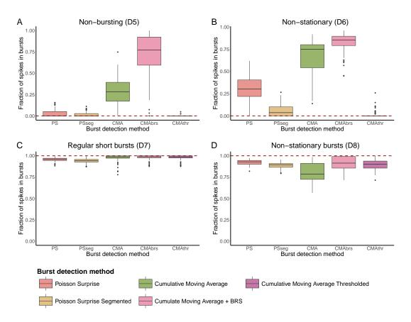
Figure 2.17: Fraction of spikes in bursts found by each burst detector in 100 synthetic trains with **A** no bursting (D5), **B** no bursting and non-stationary firing rate (D6), **C** short regular bursts (D7), **D** bursts with non-stationary burst lengths and durations (D8). Box plots and dotted line as per Figure 2.8 legend.
