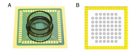
Figure 1.10: **A** A 64-channel MEA from Multi Channel Systems, and **B** configuration of the  $8 \times 8$  layout of electrodes in a 64-channel array. Standard electrode diameters are either  $10 \,\mu\text{m}$  or  $30 \,\mu\text{m}$  and the spacing of electrodes is either  $100 \,\mu\text{m}$  or  $200 \,\mu\text{m}$ . Images obtained from Multi Channel Systems MCS GmbH (2015).
