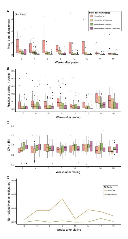
Figure 2.20: Analysis of recordings of networks of human induced pluripotent stem cell-derived neurons. A Mean burst duration, **B** fraction of spikes in bursts, and **C** coefficient of variation of interburst intervals (CV of IBI). Each data point in the box plots is the mean value across all electrodes from one recording. **D** Median normalized Hamming distance between each pairwise combination of burst detection methods at each week after plating.
