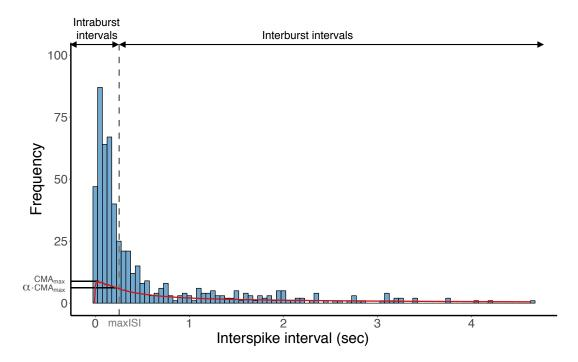
Figure 2.4: Example of ISI histogram with the threshold for intraburst and interburst intervals found using the CMA method. Red line shows the cumulative moving average of the ISI histogram.
