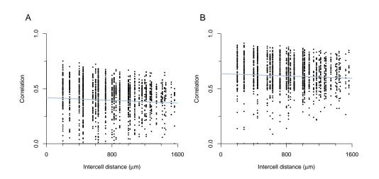
Figure 3.4: Pairwise electrode correlation values from MEA recordings from one **A** cortical and **B** hippocampal culture at 21 DIV. Blue lines show an exponential fit to the data.
