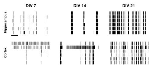
Figure 3.2: Examples of MEA recordings of spontaneous activity in one (top) hippocampal and (bottom) cortical culture at 7, 14 and 21 days in vitro (DIV). In each plot, each row is the spike train from one electrode. Six electrodes are shown from each MEA. The scale bar represents 10s of recording time. Figure reproduced from Charlesworth et al. (2015).
