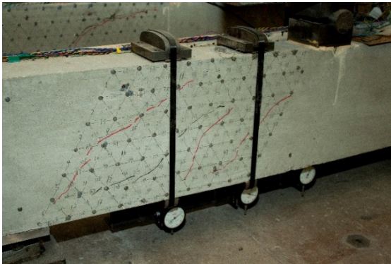
Figure 2. Photo of typical strengthened beam under sustained loading
