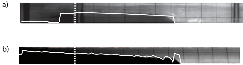
FIGURE 10. Side-view snapshots of gravity currents propagating horizontally in a) a rectangular channel and b) a V-shaped valley with tilt \phi = 45^\circ . The solid white line superimposed on both images shows the current height mid-way along the span of the tank taken from the numerical simulations at times when the computed front position is at the same location as the observed front position relative to the gate. The numerical simulations shown have g' = 4.79 \text{ cm/s}^2 , but changing the value of g' to its experimental value has very little effect on the shape of the head. The vertical dotted white line indicates the position of the gate.
