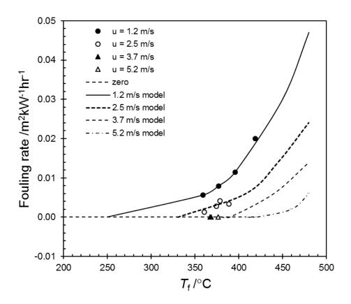
Fig. 2 The Ebert-Panchal model, Equation (1), fitted to Scarborough *et al.*'s data [6], reproduced from Ebert and Panchal [11]. Loci plotted for parameters  $a_1 = 30.2 \times 10^6$  K m<sup>2</sup>/kW h;  $b_1 = -0.88$ ,  $c_1 = 1.45 \times 10^{-4}$  m<sup>2</sup> K m<sup>2</sup>/kW Pa h and  $E_a = 68$  kJ/mol.
