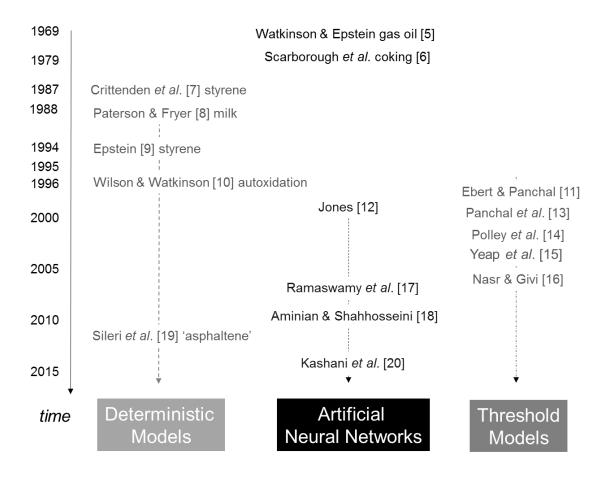
Fig. 1 Summary of quantitative chemical reaction-related fouling model studies. Left strand - deterministic models; central strand –artificial neural network approaches; right strand - threshold fouling models.
