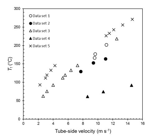
Fig. 3 Threshold fouling loci obtained by fitting the Panchal *et al.* model [13] to different sets of refinery fouling data (Labels identified in Table 1).
