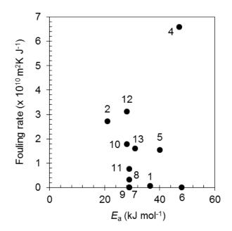
Fig. 4 Fouling rate predicted for benchmark conditions (velocity 2 m s<sup>-1</sup>, Re = 17100, Pr = 10,  $T_{\rm f} = 503$  K,  $\tau_{\rm w} = 7.2$  Pa) using the parameters reported in Table 1 (labels given in Table 1). Equation [A] predicted negative values for 6, 7 and 9 so these are plotted as zero.
