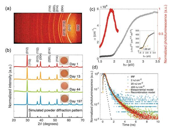
**Figure 1.** Characterization of BiOI thin films. a) 2D X-ray diffraction pattern, b) 1D X-ray diffraction patterns in ambient air over time, and c) absorption and spectrally resolved photoluminescence measurements. d) Time-correlated single photon counting measurements of BiOI in air. Biexponential and recombination models were fit to the trace measured under 400 nJ cm<sup>-2</sup> (detailed in Section S2, Supporting Information).
