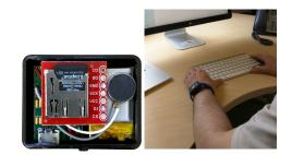
Fig. 1. Electronics (left) enclosed in 3D printed box (3x4x1.5cm) and complete prototype attached to velcro wristband (right).
