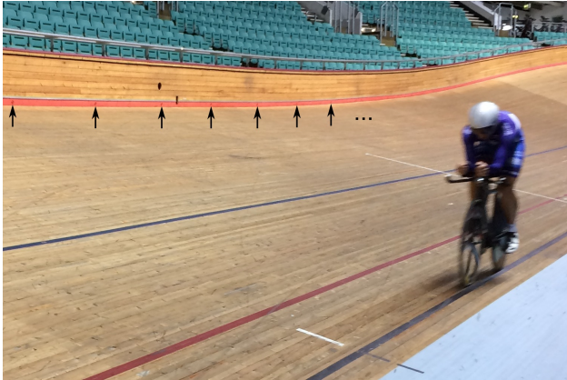
Figure 3. Cameras (arrowed) installed at two metre spacing
