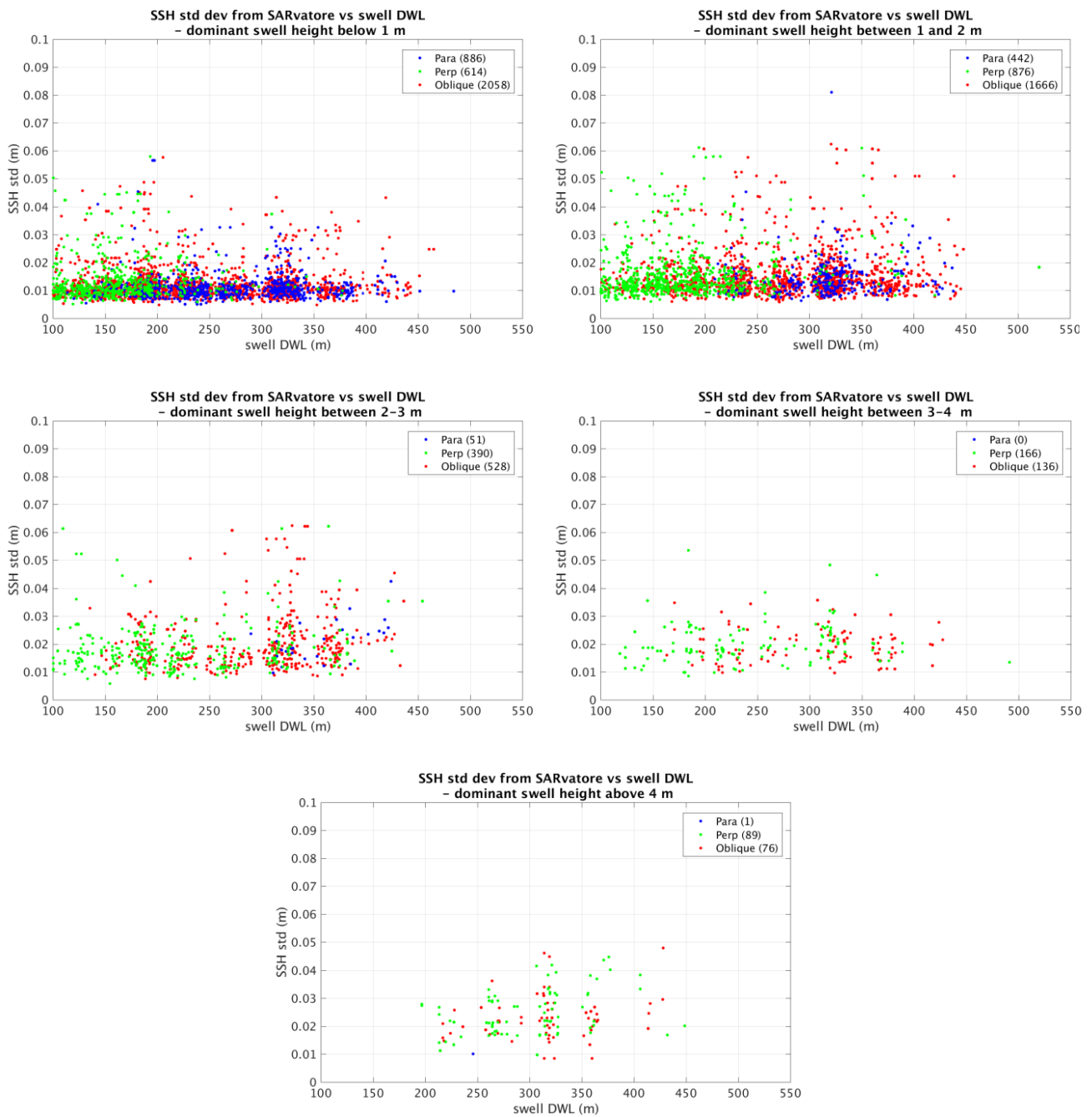
Figure 33: Cryosat-2 SAR SSH variability (20Hz std) against Envisat ASAR dominant wave length, plotted for different dominant swell height categories, for (blue) parallel, (green) perpendicular and (red) oblique swell orientation.
