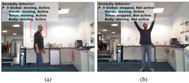
Fig. 2: Results of activity level detection when the person is (a) walking and (b) moving his arms.
