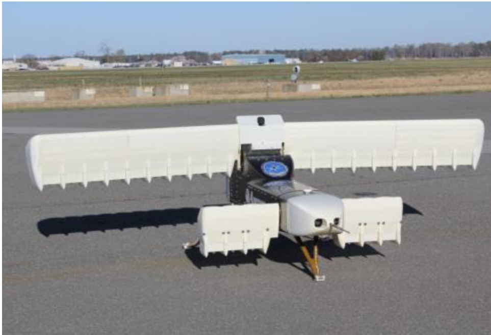
Figure 9. Hence, 24 engine nacelles were designed within in-wing motor compartments [100, 101].
