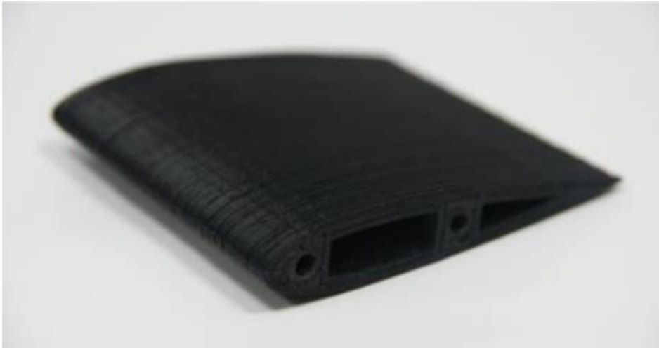
Figure 12 [110] . By adopting FDM, it was possible to improve computational fluid dynamics, and validate the models experimentally using FDM parts in wind tunnels.
