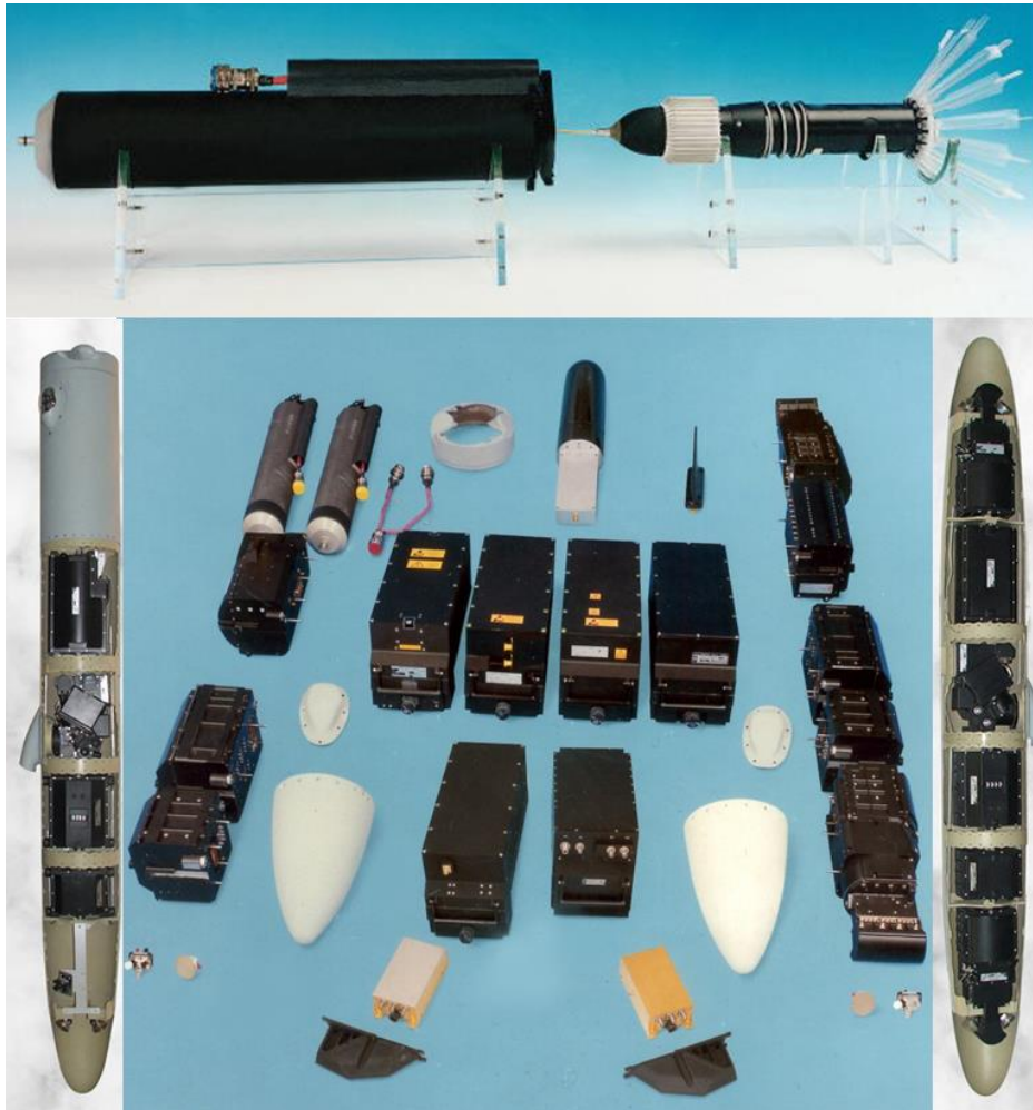
Figure 3. Typhoon's Praetorian Defensive Aids Sub-System (© Leonardo MW Ltd 2016 All rights reserved)
