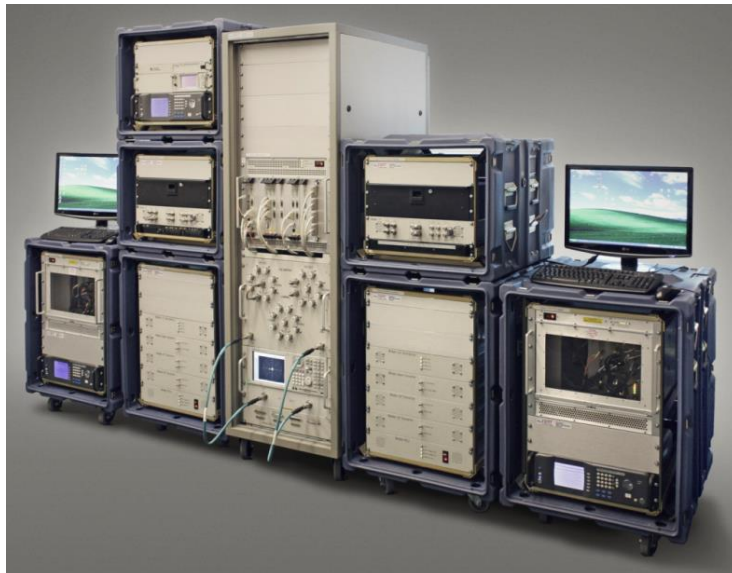
Figure 27. Chameleon II radar target and ECM simulator (© Ultra Electronics Ltd. 2014)
