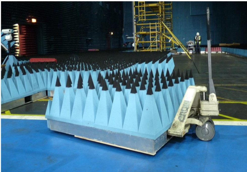
Figure 37. Chamber floor RAM pallet and mover (© 2016 BAE SYSTEMS. All rights reserved.)
