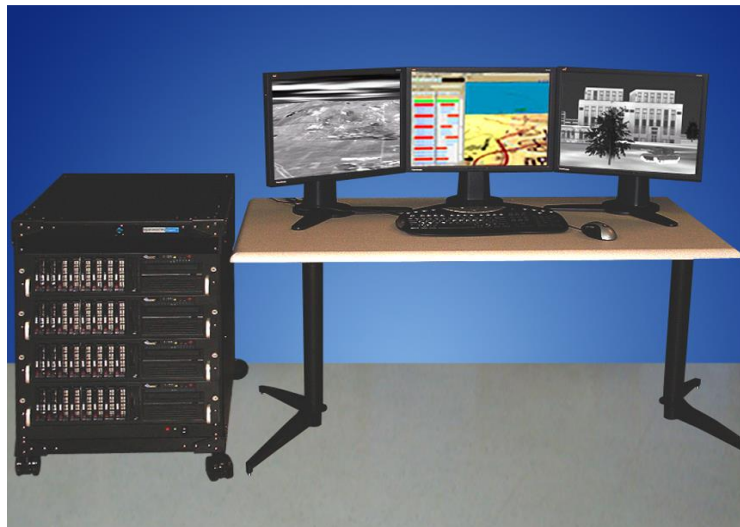
Figure 42. IR scene simulator - RISS (© Northrop Grumman – Amherst Systems 2016)
