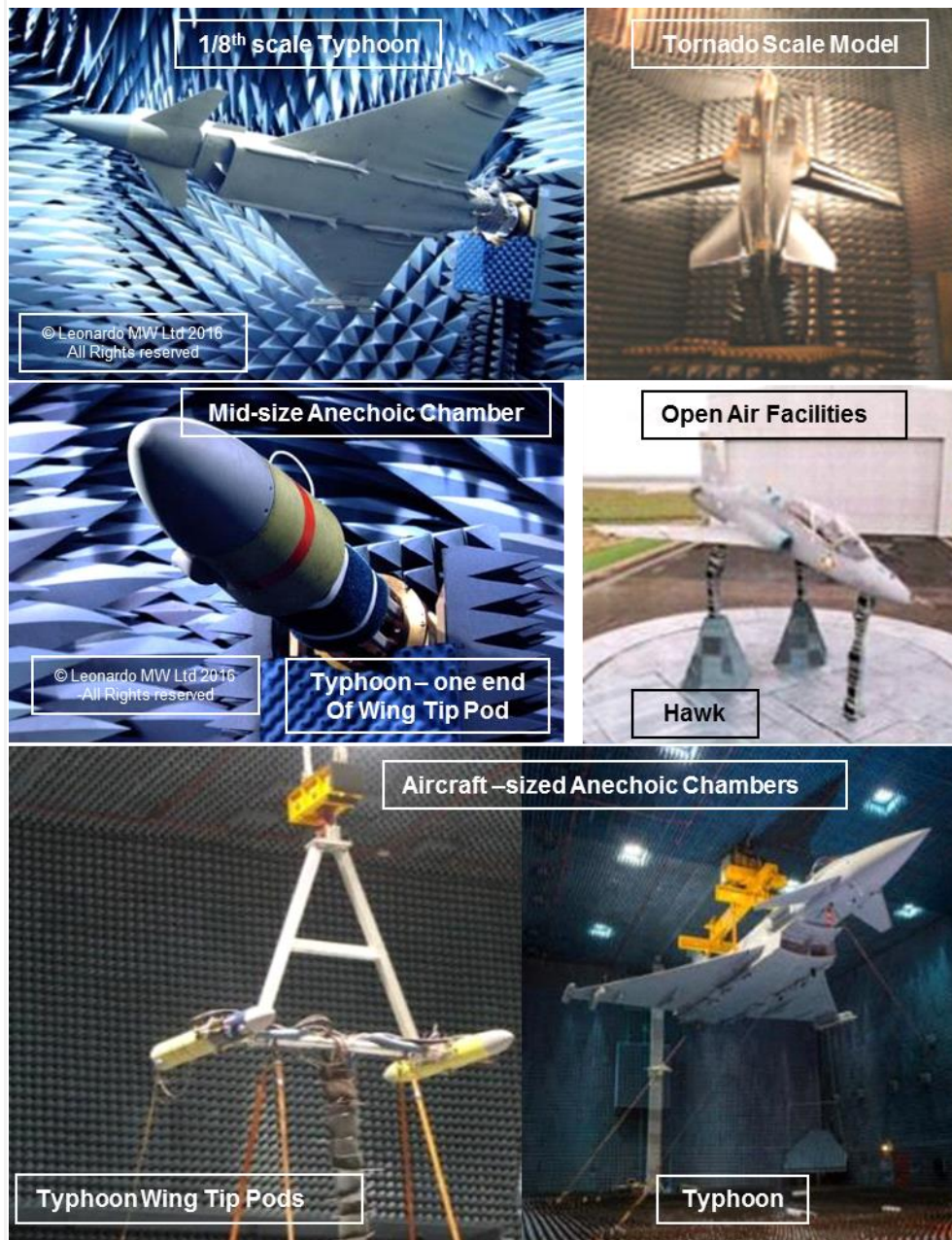
Figure 33. Antenna pattern measurement facilities (Except Leonardo images, © 2016 BAE SYSTEMS. All rights reserved.)
