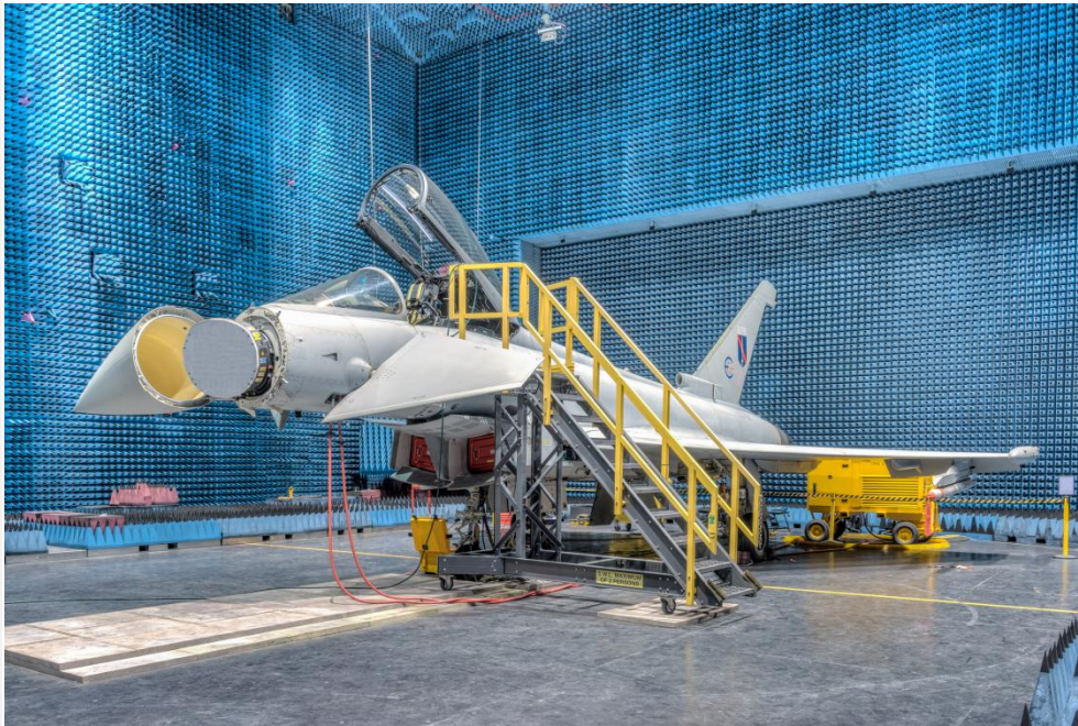
Figure 29. Typhoon E-Scan radar and DASS tests in EWTF (© 2016 BAE SYSTEMS. All rights reserved.)
