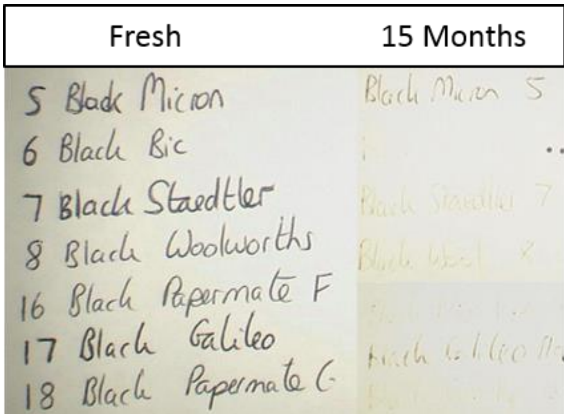
Figure 5.5 Image of Fresh Black Ink and ink exposed to daylight for 15 months
