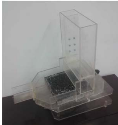
(b) Photograph of permeameter
