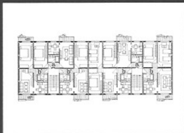
Fig. 3. A floor plan of a housing block in Karpoš built from prefabricated panels, a) two-room apartment-47.77 m 2 , b) two room apartment 51.07 m 2 , c) three room apartment 69.28 m 2
