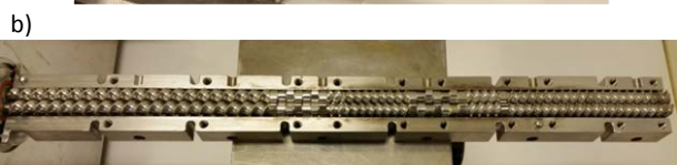
Figure 1: a) Twin screw extruder and b) intermeshing co-rotating screws encased in the extruder barrel.
