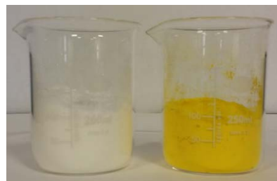
Figure 4: Mixture of vanillin and barbituric acid before extrusion (left) and the extruded product, 1a (right).
