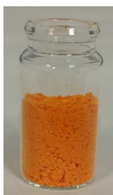
Figure 17: Orange solid ( 4 ) produced from the twin screw extrusion of 4,4'-oxydianiline and 2 equivalents of ortho -vanillin.
