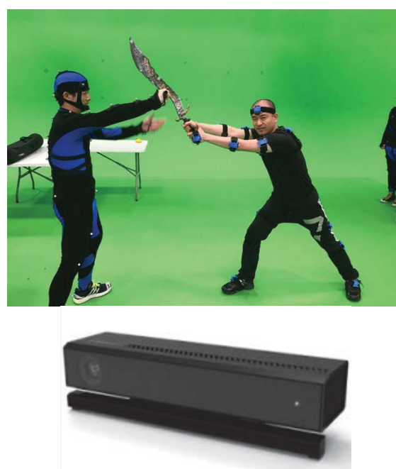
Fig. 1: Examples of MOCAP equipments: (1) optical based (upper left), (2) wearable sensors (upper right) and (3) depth sensors (bottom)
