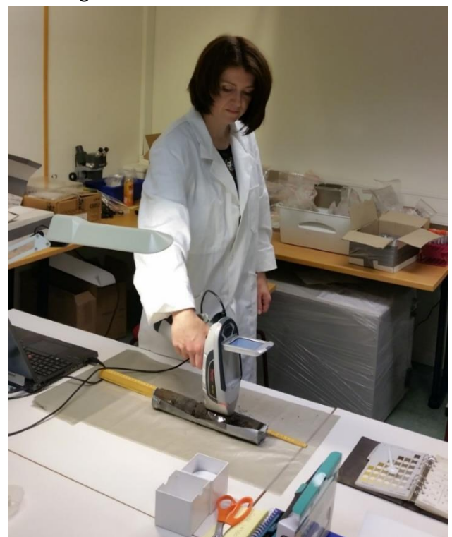
Figure 4. 9. An opened core being directly analysed using pXRF. Photo: Marianne Hem Eriksen/author.
