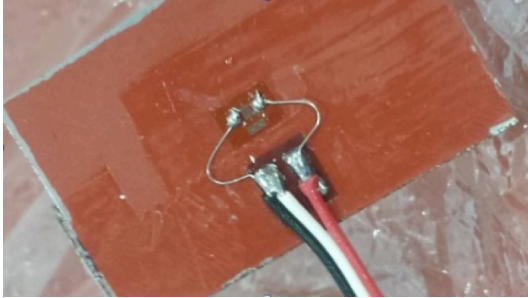
Figure 2 Strain gauge mounted on coating/substrate system
