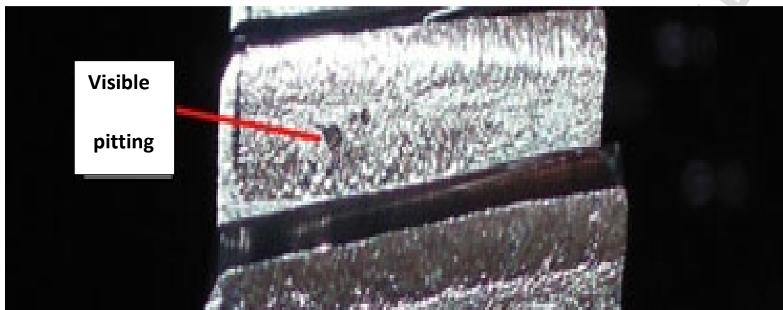
Figure 12 Visible pitting after test 1 [50]
