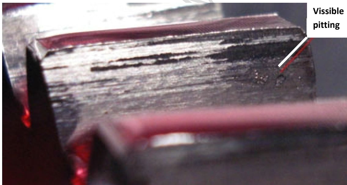
Figure 13 Visible damage after test 2 [50]
