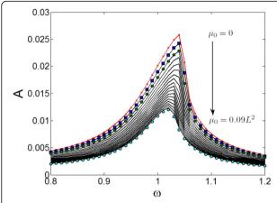
**Fig. 3** Calculated non-dimensionalised displacement versus the driving frequency of the nanowire resonator
