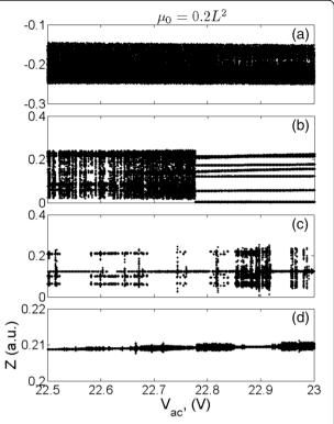
**Fig. 5** Bifurcation analysis of the resonator without considering the nonlocal effect. **a** The frequency ratio  $\omega/\omega 0$  is 0.8. **b** The frequency ratio  $\omega/\omega 0$  is 1. **c** The frequency ratio  $\omega/\omega 0$  is 1.1. **d** The frequency ratio  $\omega/\omega 0$  is 1.2.
