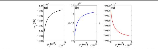
Fig. 2 The calculated results of resonate frequency  $\omega_0$  (a), Duffing coefficient  $\beta$  (b), and damping ratio  $\gamma$  (c) related to the nonlocal coefficient  $\mu_0$
