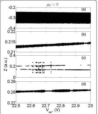
**Fig. 6** Bifurcation analysis of the resonator considering the nonlocal effect. The frequency ratio  $\omega/\omega 0$  is 0.8 (a), 1 (b), 1.1 (c), and 1.2 (d)
