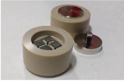
Fig. 2. Picture of the evaluated multiple and single chip SiC Schottky diode modules using pressure contacts in different assembly stages
