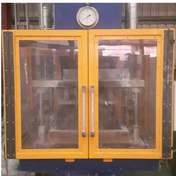
Figure 8 – Press used to form VIP core shape via load application
