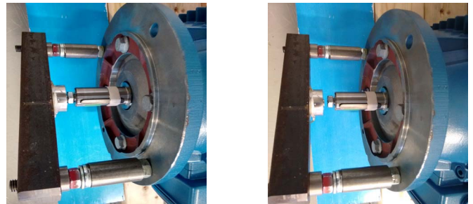
a) End-stop plate allows 0 mm axial movement b) End-stop plate allows 4 mm axial movement
