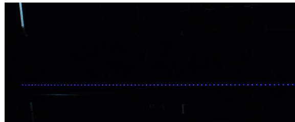
Figure 4 A photo of glow discharges from the actuator.
