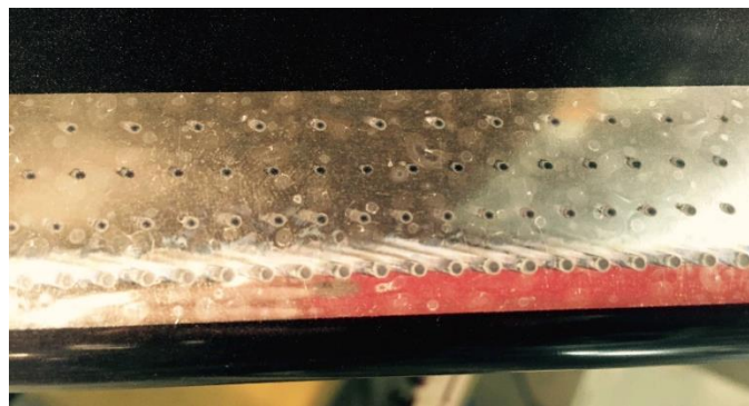
Figure 12 Stains left on the actuator sheet after wind tunnel tests.
